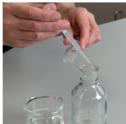
Photo 3. Adding a few drops of aqueous sodium thiosulphate solution
