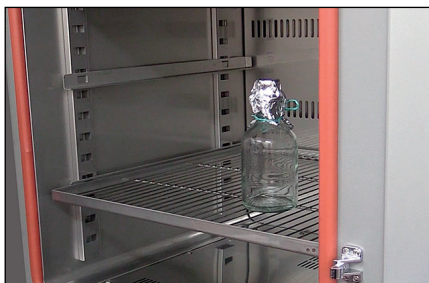
Photo 7. Sterilization in an oven
