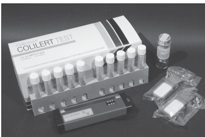
Colilert test, H 2 S strip and dipslides
