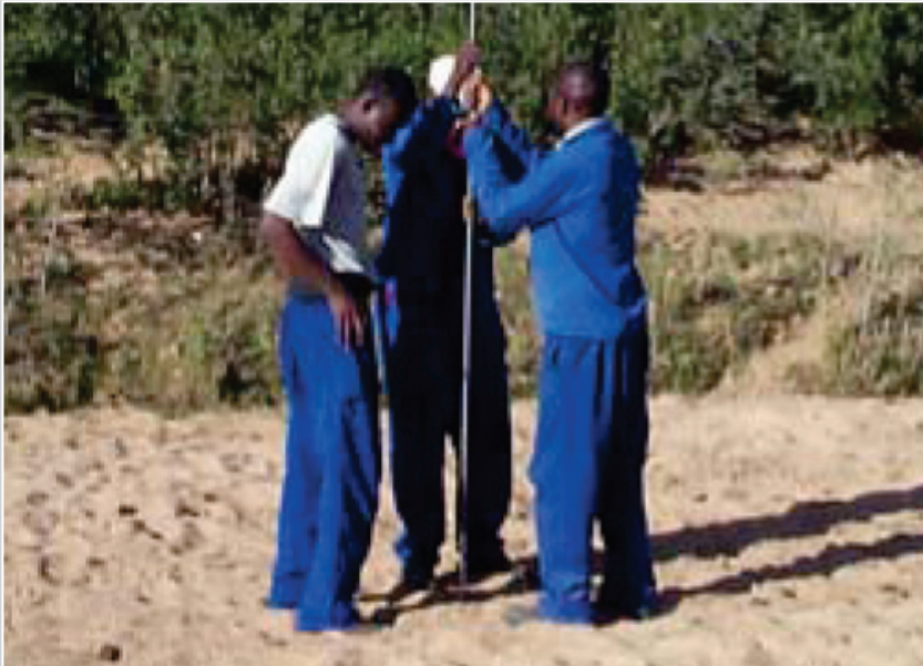
Photograph 3.5. Establishing the depth of sediment with a probe
