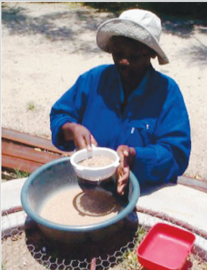
Photograph 3.8. Simple grading test using household sieve
