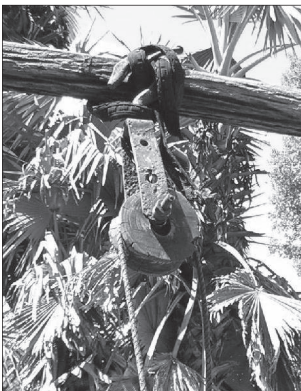
Figure 6.8. Detail of pulley lifting mechanism. (Case-study 9.12, page 191)
