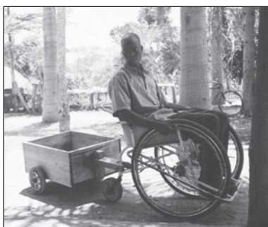
Figure 9.150. Two-wheeled wooden trailer.
