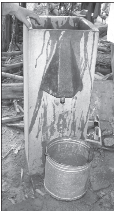
Figure 9.59. Sand water filter.
