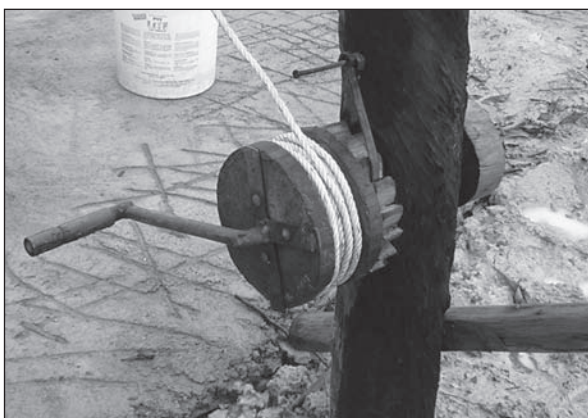
Figure 6.9. Detail of ratchet and pawl winding mechanism.
