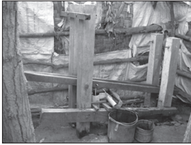
Figure 9.55. Treadle pump.
