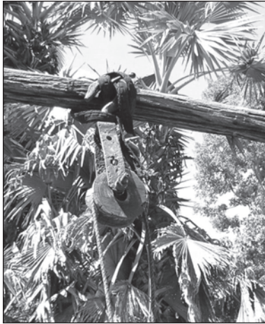
Figure 9.52. Locally made wood and metal pulley.
