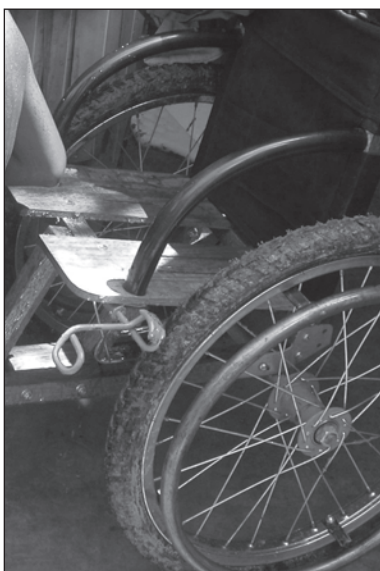
Figure 9.75. Wheelchair seat with central plank removed.
