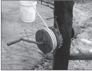
Figure 9.49. Ratchet and pawl locking mechanism. The metal pawl is engaged with the notches of the ratchet to prevent onward movement.
