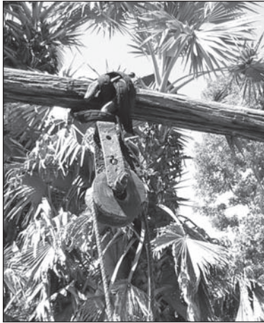
Figure 9.52. Locally made wood and metal pulley.
