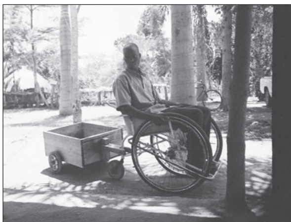
Figure 6.29. Two-wheeled wooden wheelchair trailer.
