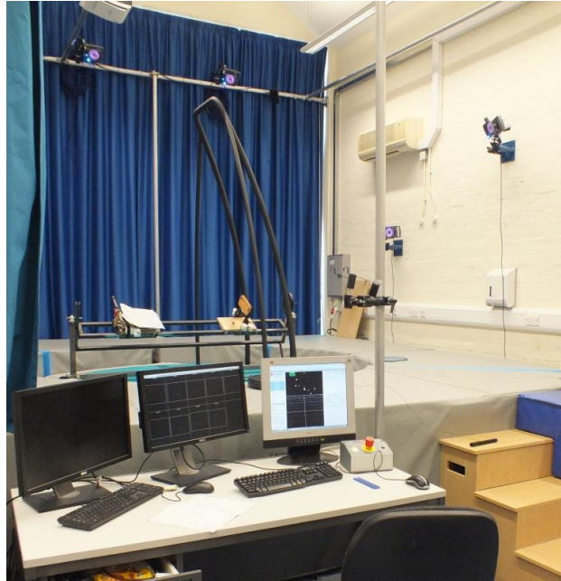
Figure 6-5: Vicon system set-up integrated within CAREN laboratory.
