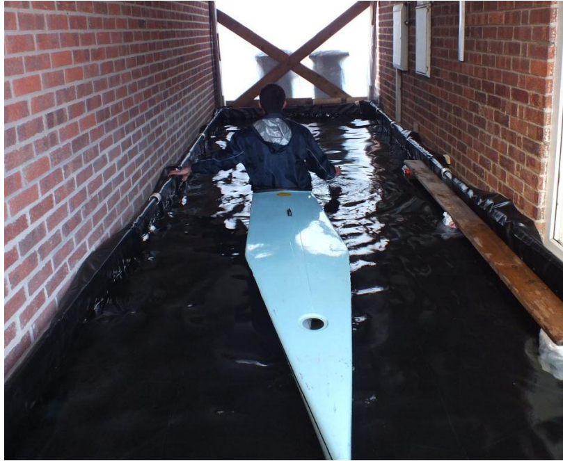
Figure 6-2: On-water training and assessment pool (Width – 1.5 m; Length – 6.0 m; Depth – 0.30 m).
