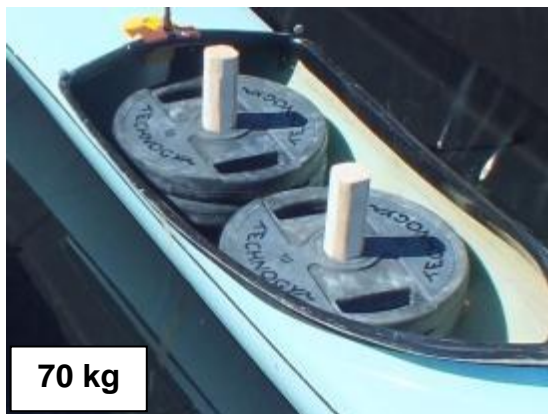
Figure 5-3: Additional weight positioning for the on-water medial-lateral rolling analysis.
