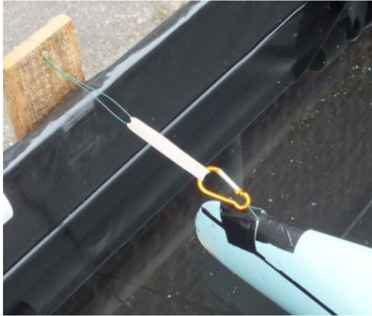
Figure A5-2: Anchor system to minimise sway motion.
