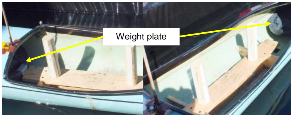
Figure 5-2: Weight plate positioning of the initial 30 kg (3 plates) additional weight.
