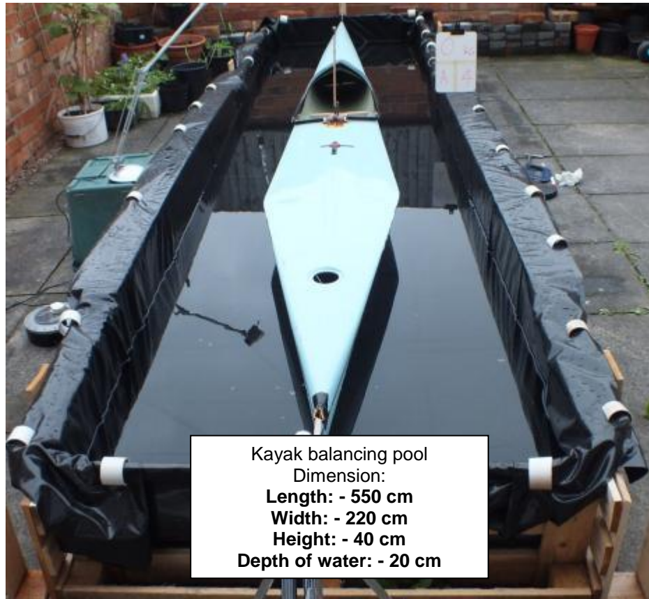
Figure A5-1: Kayak balancing pool set-up for oscillation test.
