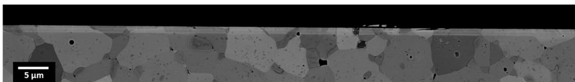
**Figure 107** Photo montage showing the consistency of the ion damage layer across the sample.
