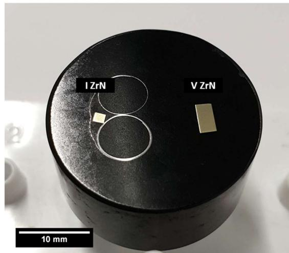
*Figure 53 Mounted samples of irradiated and unirradiated ZrN.*
