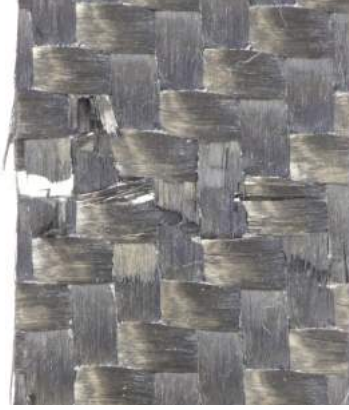
Figure 8.2: CFRP tensile test specimen - tensile fibre damage
