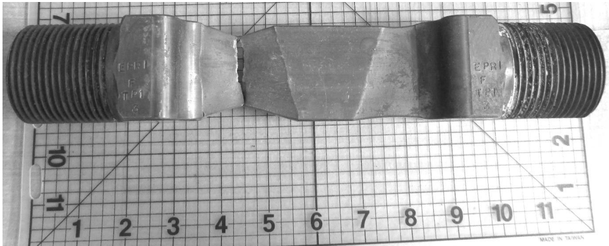
Figure 6-11. Example of parent metal dominated failure (sample F-TP1-3)
