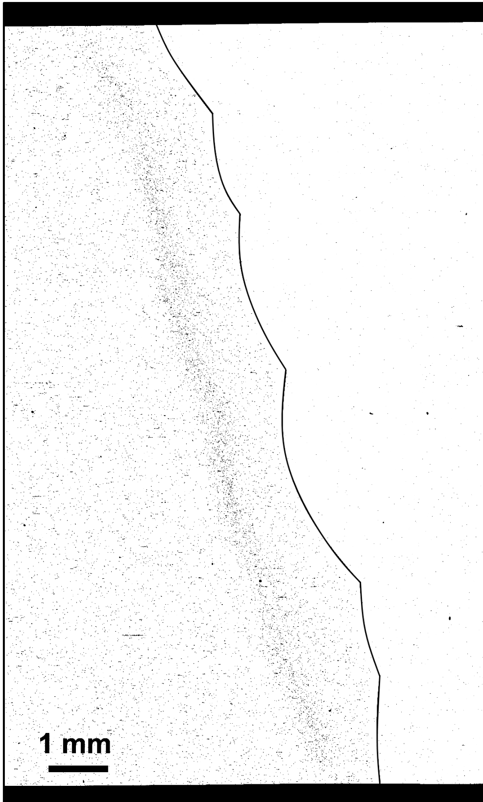
Figure 4-23. The distribution of damage through the heat affected zone in the interrupted sample RND-B2-1 (12.7 mm diameter, 1,347 hours to termination, 64% time fraction, 85% strain fraction).
