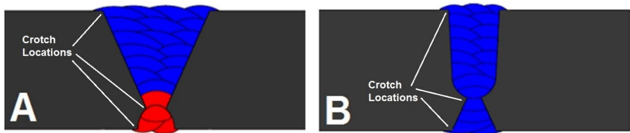
Figure 2-25. Difference in performance of seam welded Grade 91 type components have been recorded during service. Damage and cracking were found in elbows which had been made using a high bevel angle (A) rather than in straight pipe sections where the weld profile was significantly different (B) (Komai 2016)
