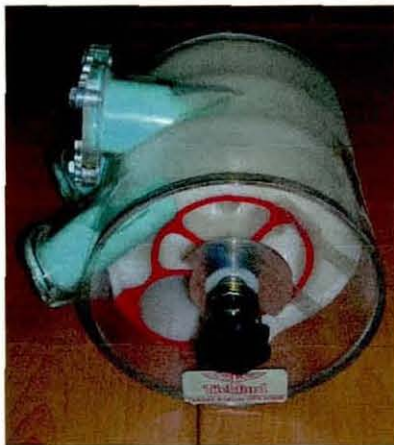
(a) End view showing primary inlet runner
