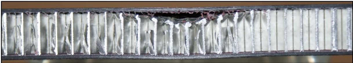
Figure 4.2.10. Cross section of thin symmetrical CP carbon/epoxy panel with 135 kg/m<sup>3</sup> core density impacted at 20J
