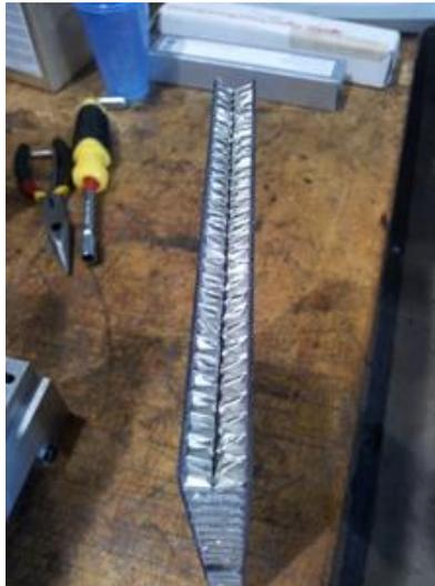
**Figure 5.1.2. Photo of V-notch cut into top of panel to improve epoxy penetration**
