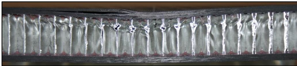
Figure 4.2.6. Cross section of thick symmetrical CP carbon/epoxy panel with 70 kg/m<sup>3</sup> core density impacted at 45J
