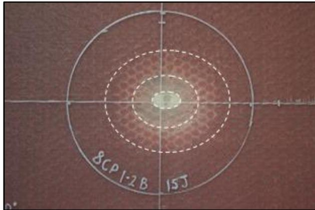
**Figure 4.1.5. Impact damage in a thin symmetrical CP E-glass/epoxy panel with 70kg/m<sup>3</sup> core impacted at 15J as seen through the skin surface (SG-8-8-CP-15J)**
