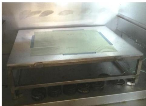
Figure 2.3.2. Oven table with bagging release film tapped down ready for skin/core bonding
