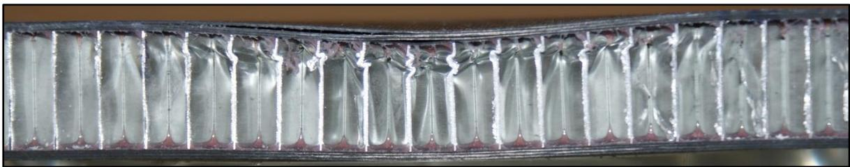
Figure 4.2.2. Cross section of thin symmetrical CP carbon/epoxy panel with  $70\text{ kg/m}^3$  core density impacted with 16J
