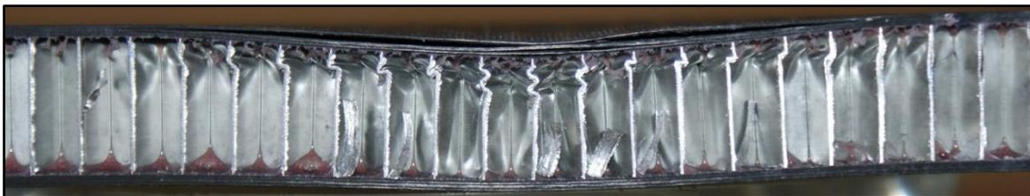
Figure 4.2.3. Cross section of thin symmetrical CP carbon/epoxy panel with  $70\text{ kg/m}^3$  core density impacted with 23J
