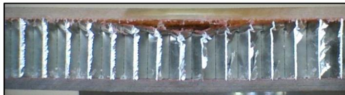
(c) Thin symmetrical CP E-glass/epoxy panel with 70kg/m<sup>3</sup> core density impacted at 18J (SG-16-16-CP-18J-B)
