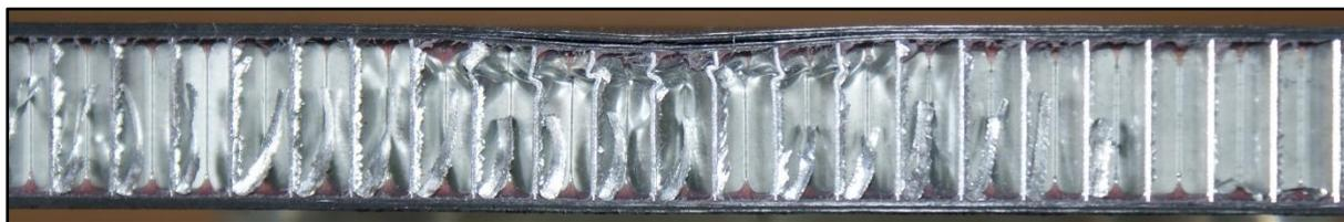
**Figure 4.1.1. Cross section of a thin unsymmetrical CP carbon/epoxy panel with 70kg/m<sup>3</sup> core density impacted at 5J (DJ-8-6-CP-5J-B1)**
