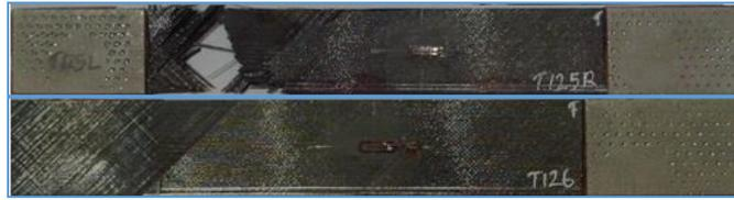
**Figure 2.1.2. Failed specimens T125 and T126 showing premature failure modes (a) failure near end tab (b) top ply sheared off under tab**
