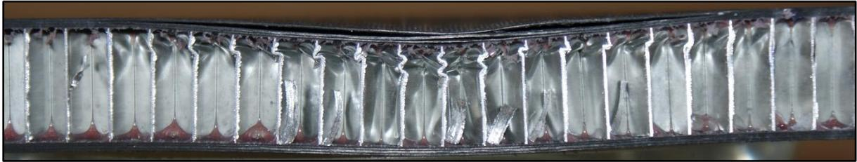
Figure 4.1.2. Cross section of a thin symmetrical CP carbon/epoxy panel with 70kg/m<sup>3</sup> core density impacted at 23J (CI-8-8-CP-23J-B)
