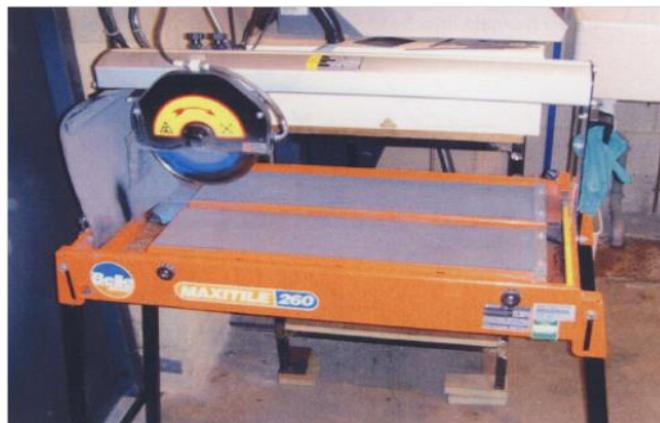
**Figure 2.2.10. Diamond edged radial saw**
