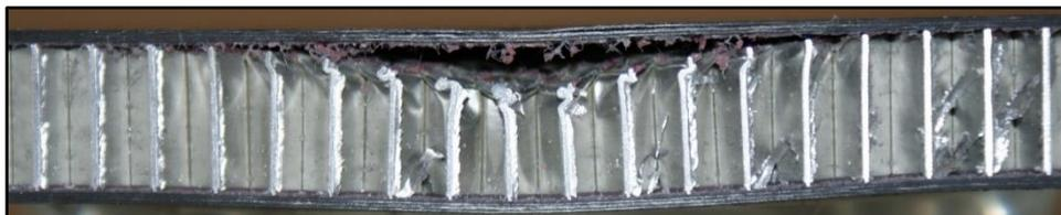
(b) Thin symmetrical CP carbon/epoxy panel with 135kg/m<sup>3</sup> core density impacted at 45J (RM-8-8-CP-40J-B)
