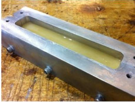
**Figure 5.1.1. Photo of end potting mould with epoxy resin inside**
