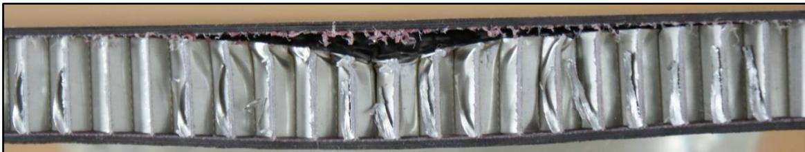
Figure 4.2.11. Cross section of thin symmetrical CP carbon/epoxy panel with 135 kg/m<sup>3</sup> core density impacted at 30J
