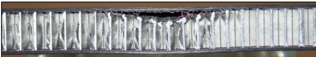
(a) Thin symmetrical CP carbon/epoxy panel with 135kg/m<sup>3</sup> core density impacted at 20J (RM-8-8-CP-20J-B)
