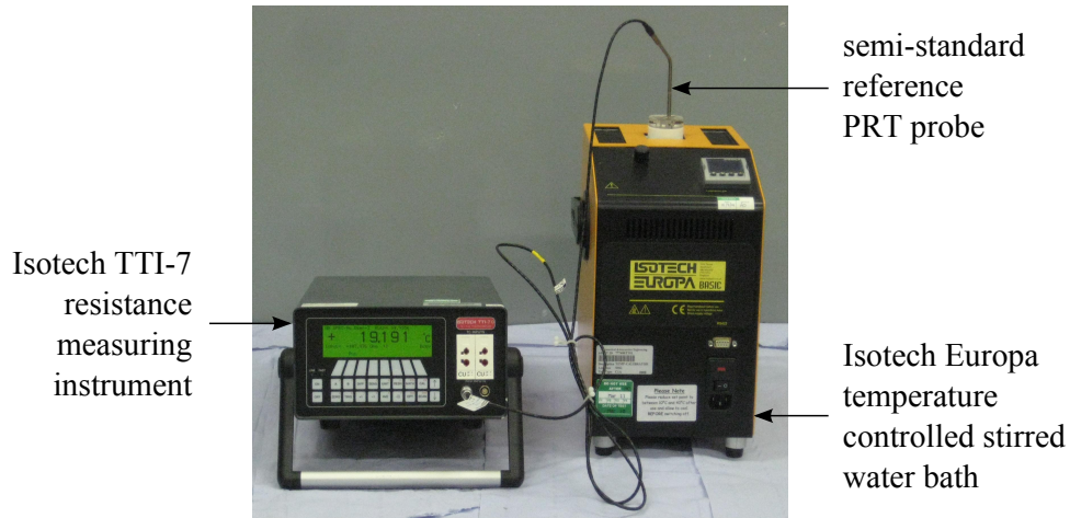
Figure 3.7: Temperature probe calibration equipment.
