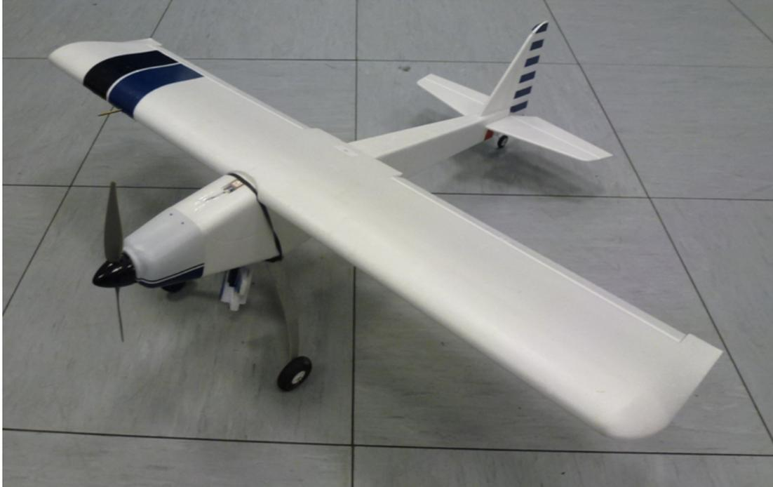
Figure 6.8: Ripmax Wot4 Foam-E with [APM](#) installed
