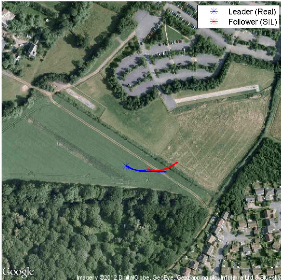
Figure 6.13: Mixed mode (SIL and real) formation flight
