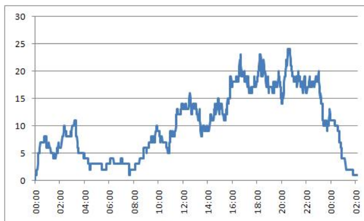
Figure 7.4: Demand profile created for the City BCU of Leicestershire using enhanced probabilistic approach.
