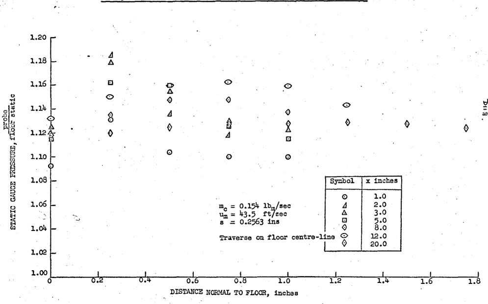
FIG. 9.8: NORMAL STATIC PRESSURE GRADIENTS AT DOWNSTREAM LOCATIONS
