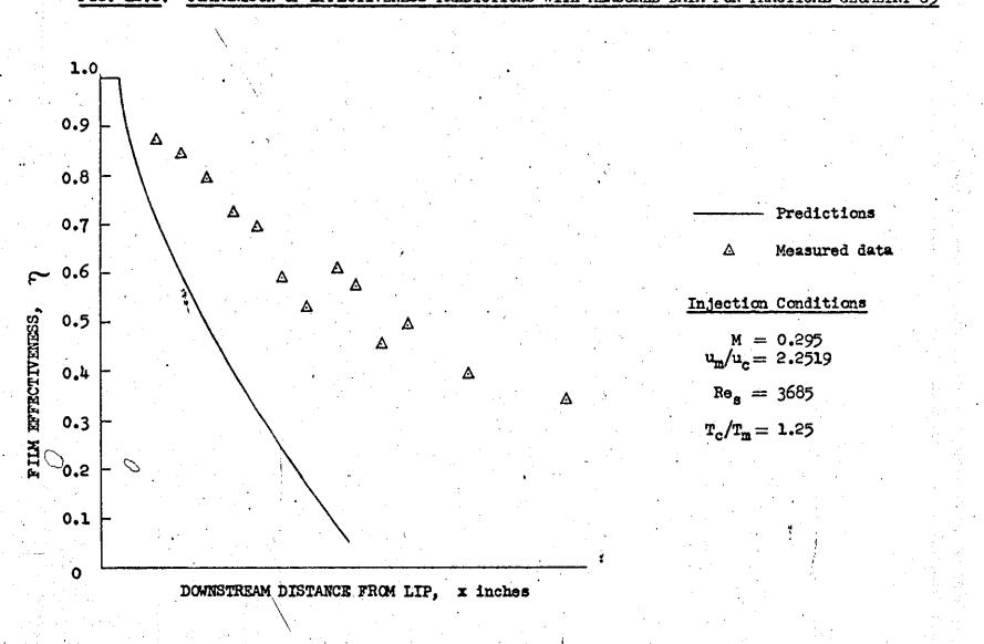
FIG. 12.6: COMPARISON OF EFFECTIVENESS PREDICTIONS WITH MEASURED DATA FOR PRACTICAL GEOMETRY G5
