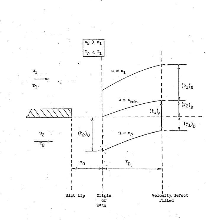
FIG. 7.4: FILLING OF VELOCITY DEFECT
