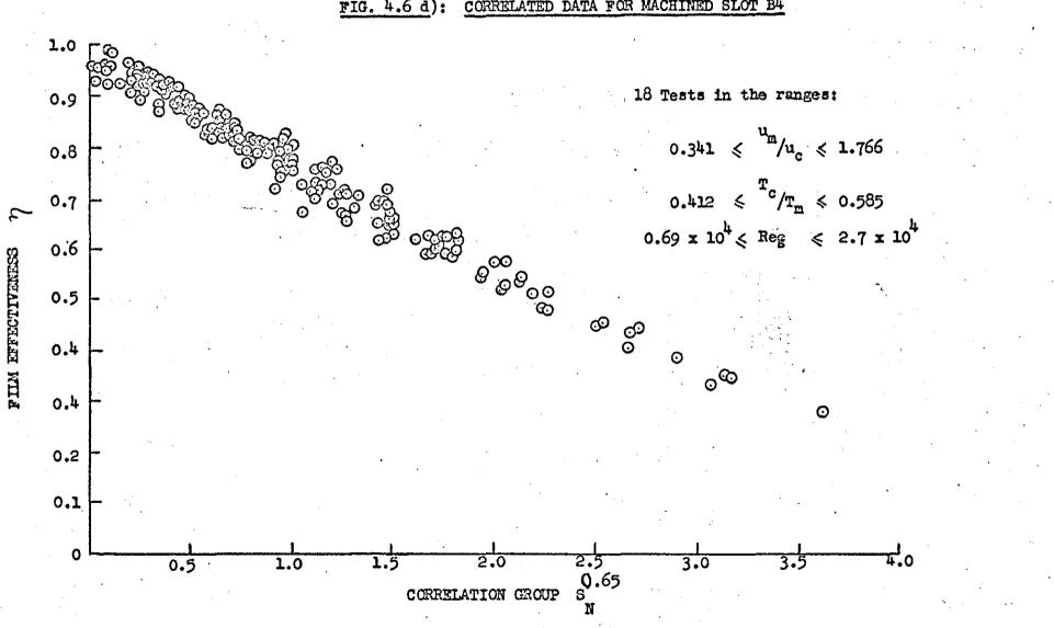
FIG. 4.6 d): CORRELATED DATA FOR MACHINED SLOT B4
