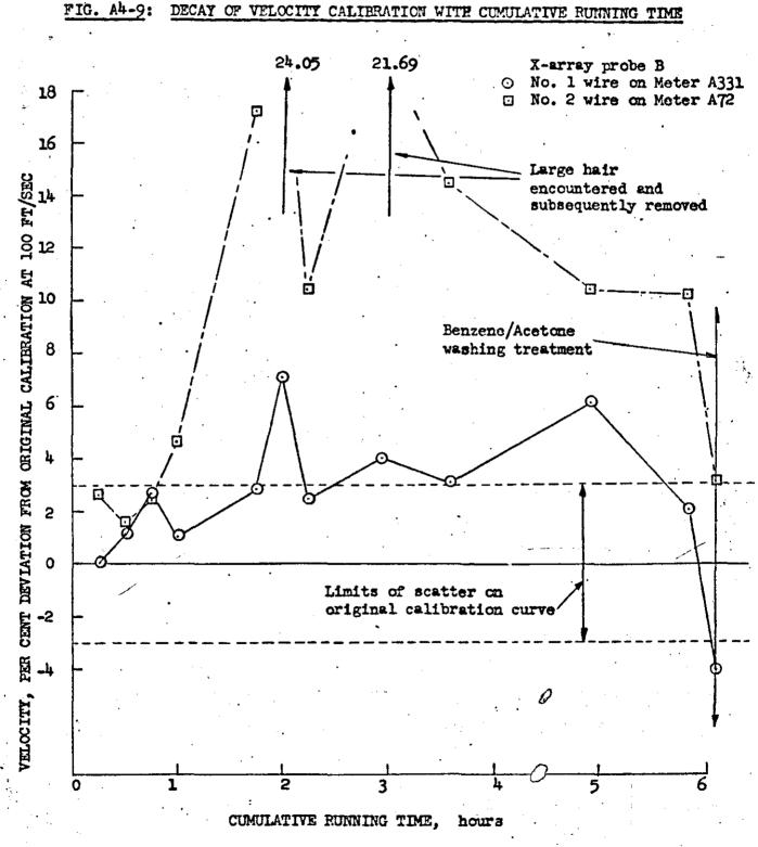
DECAY OF VELOCITY CALIBRATION WITH CUMULATIVE RUNNING TIME
