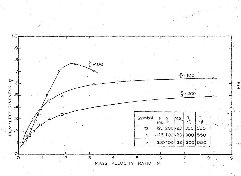
FIG. 2.12: EFFECT OF MASS VELOCITY RATIO ON EFFECTIVENESS USING PAPELL AND TROUT'S DATA
