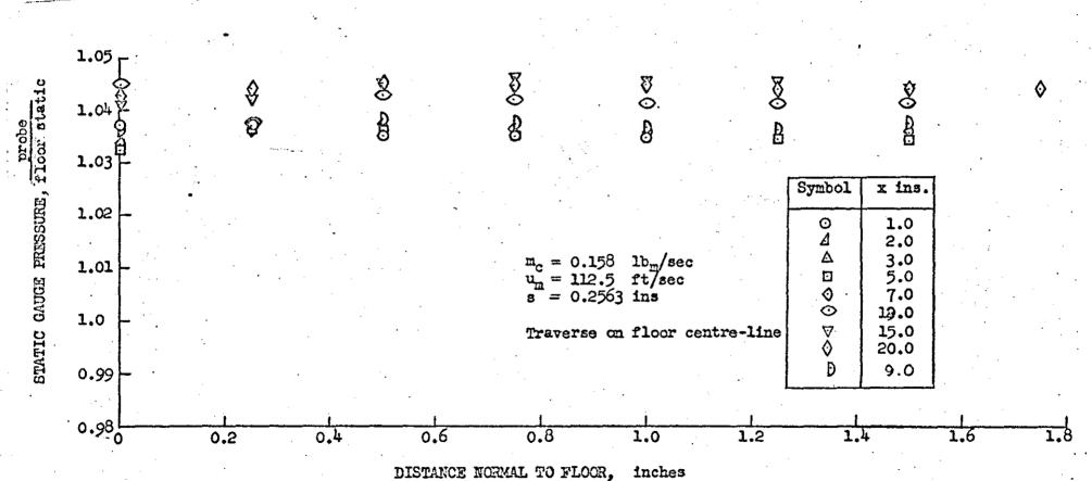
FIG. 9.7: NORMAL STATIC PRESSURE GRADIENTS AT DOWNSTREAM LOCATIONS
