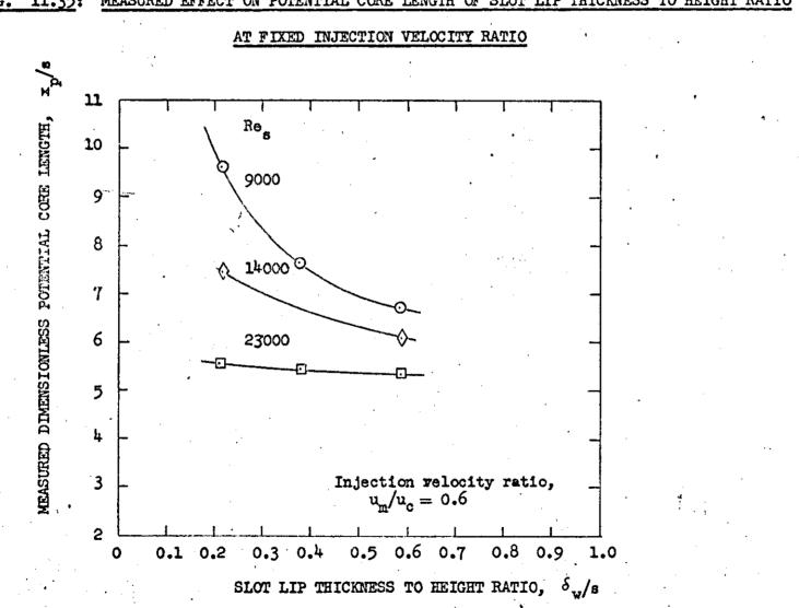
MEASURED EFFECT ON POTENTIAL CORE LENGTH OF SLOT LIP THICKNESS TO HEIGHT RATIO FIG. 11.35:
