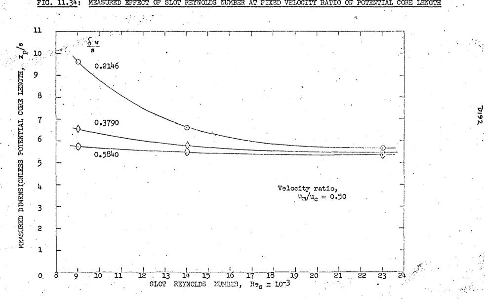
FIG. 11.34: MEASURED EFFECT OF SLOT REYNOLDS NUMBER AT FIXED VELOCITY RATIO ON POTENTIAL CORE LENGTH
