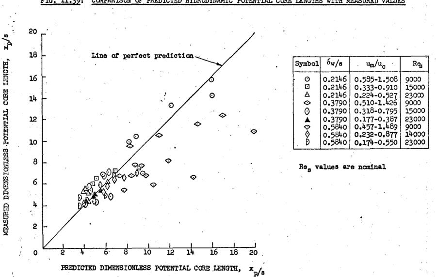
FIG. 11.39: COMPARISON OF PREDICTED HYDRODYNAMIC POTENTIAL CORE LENGTHS WITH MEASURED VALUES
