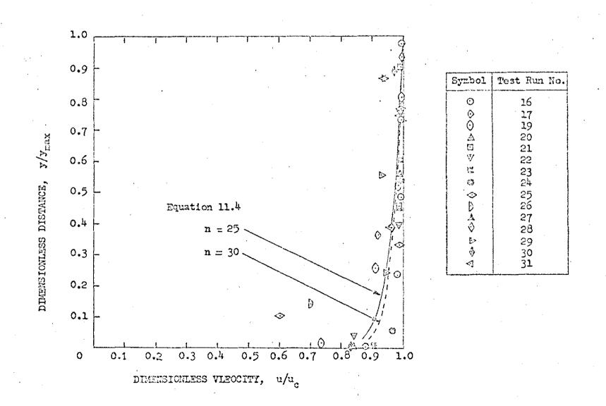
FIG. 11.21: UNIVERSAL VELOCITY FROFILE FOR SLOT LIP INNER BOUNDARY LAYER - THIN LIPPED SLOT
