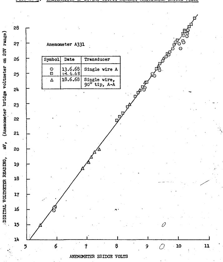
FIG. A4-3: CALIBRATION OF D.V.M. OUTPUT AGAINST ANEMOMETER BRIDGE VOLTS
