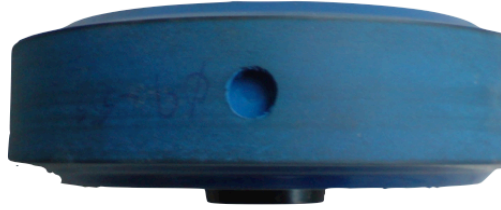
Figure 7.1 Photograph of top view of the tyre equipped with the 'large cavity'
