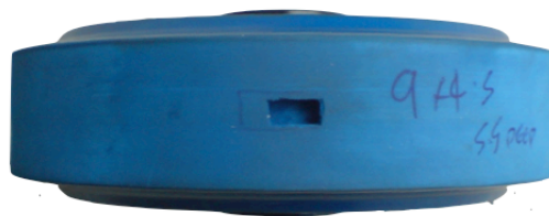
Figure 7.16 Photograph of top view of the tyre equipped with the 'long cavity'
