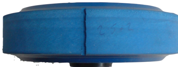
Figure 6.9 Photograph of top view of the tyre equipped with the 'small groove'
