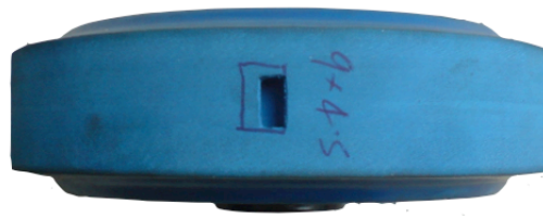
Figure 7.20 Photograph of top view of the tyre equipped with the 'wide cavity'
