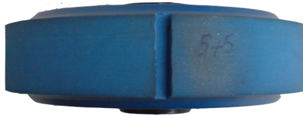
Figure 6.1 Photograph of top view of the tyre equipped with the 'square groove'
