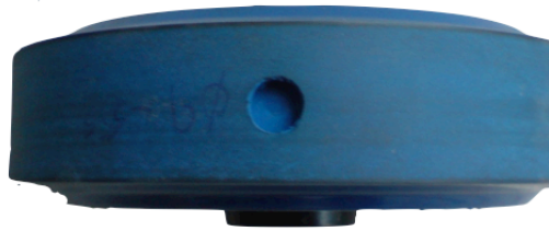
Figure 5.5 Photograph of top view of the tyre equipped with the 'large cavity'
