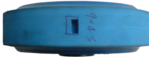
Figure 5.32 Photograph of top view of the tyre equipped with the 'wide cavity'
