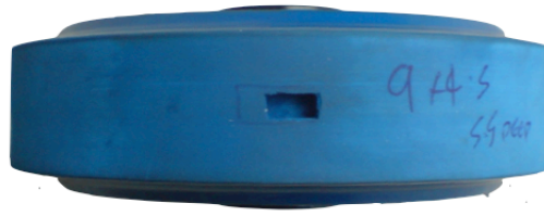
Figure 5.26 Photograph of top view of the tyre equipped with the 'long cavity'
