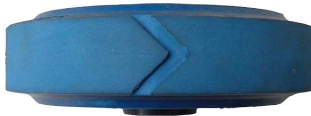
Figure 6.16 Photograph of top view of the tyre equipped with the 'chevron' shape of groove
