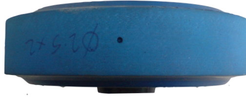
Figure 5.13 Photograph of top view of the tyre equipped with the 'small cavity'
