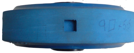
Figure 5.19 Photograph of top view of the tyre equipped with the 'square cavity'
