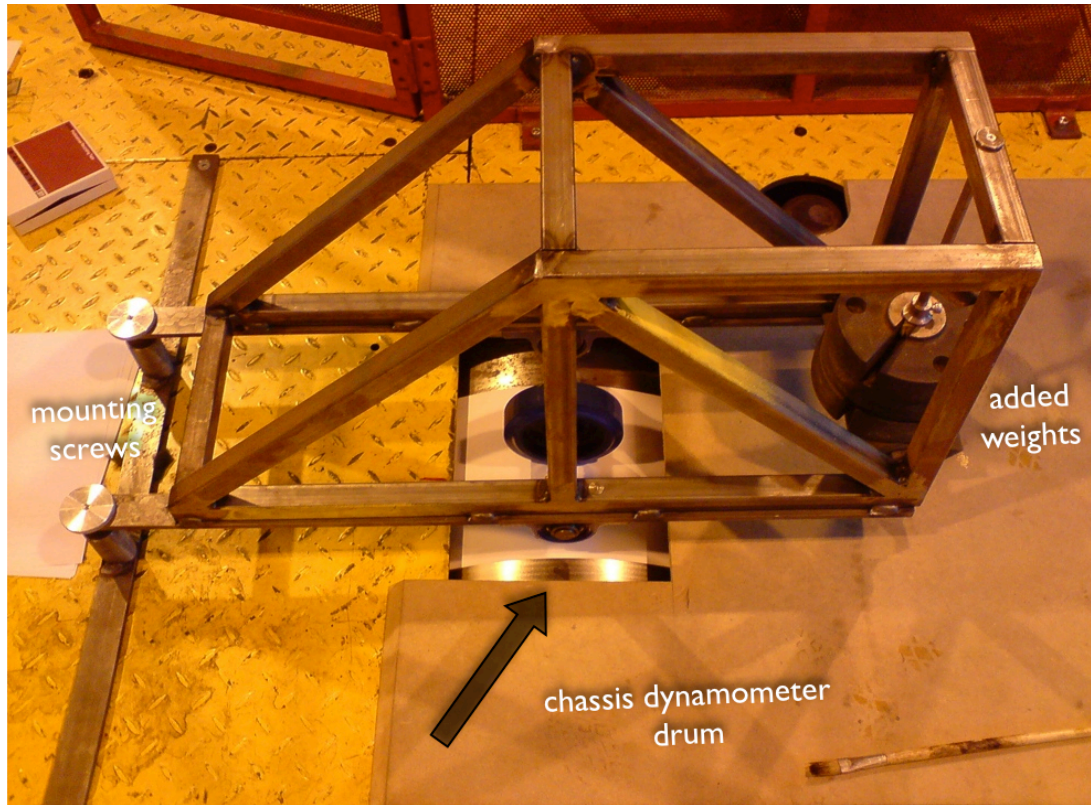
Figure 4.10 Photograph of the original rig layout with tyre, wooden cover and weights in place
