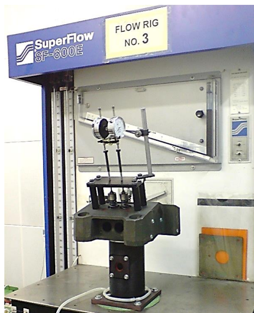
Figure 4-7 Steady Flow rig
