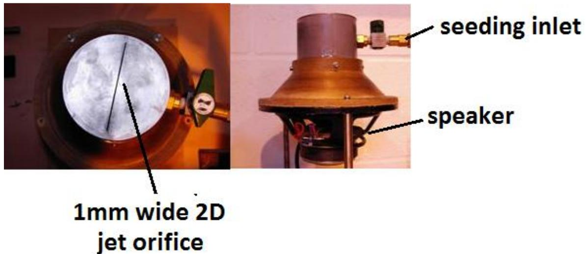
**Figure 4.7 - Speaker driven SJ rig for time resolved PIV studies**
