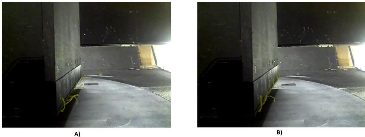
**Figure 6.8 – Images of wool tufts at slot exit for configuration D, for A) valve closed state B) valve closed state**
