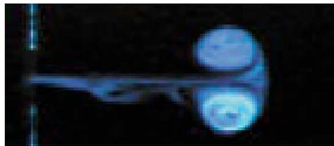
**Figure 4.2 - Synthetic jet with characteristic vortices (Glezer and Amitay, 2002)**
