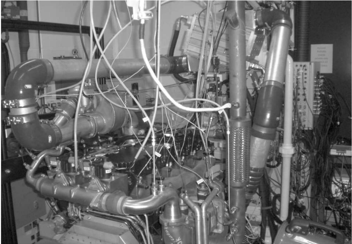
**Figure 5.8:** Test cell arrangement at Loughborough University for the Caterpillar C6.6 medium-duty engine.
