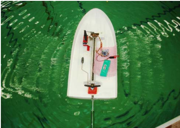
Fig.5 Static thrust test in progress
