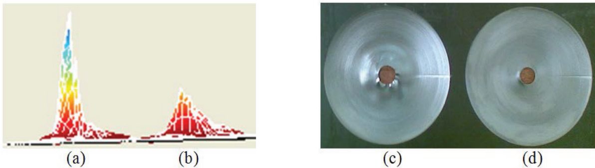
Figure 10 - (a) Displacement of the indentation shown in c, (b) Displacement of the indentation shown in d, (c) Circular indentation with a thinner damaged tip, (d) Circular indentation with a thicker undamaged tip
