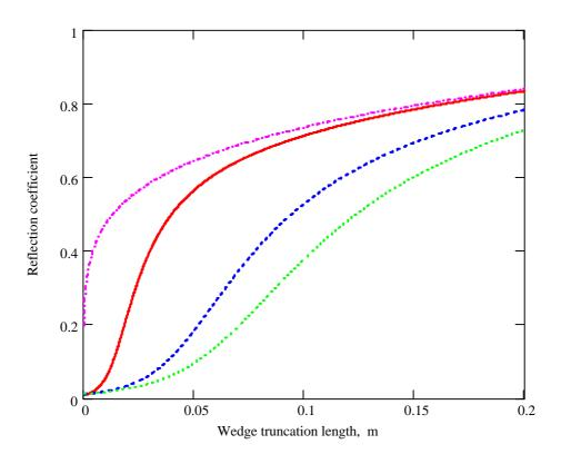
Figure 8. Reflection coefficient for the wedge covered by a thick absorbing film: the values of film thickness  $\delta$  are: 10  $\mu m$  (solid curve), 100  $\mu m$  (dashed curve) and 200  $\mu m$  (dotted curve), dash-dotted curve shows the behaviour of the reflection coefficient for the uncovered wedge; other parameters of the wedge and film are the same as on Figure 7.
