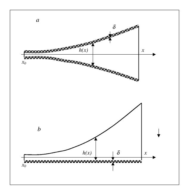
Figure 2. Truncated quadratic wedges covered by thin damping layers: *a*) Symmetric wedge covered on both sides; *b*) Non-symmetric wedge that is covered on one side only.
