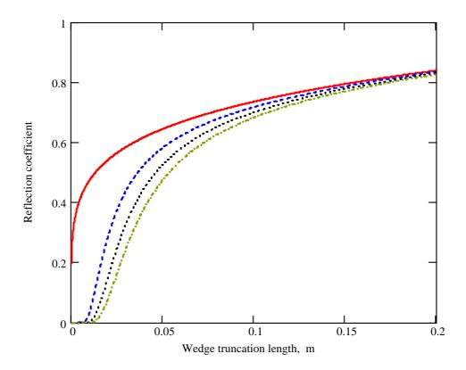
Figure 4. Effect of wedge truncation length  $x_0$  (in m) on the reflection coefficient  $R_0$ : solid curve corresponds to an uncovered wedge, dashed, dotted and dash-dotted curves correspond to a wedge covered by absorbing films with the values of relative film stiffness  $E_2/E_1$  equal to 0.1, 0.2 and 0.3 respectively; the film material loss factor v is 0.15, and the film thickness  $\delta$  is 15  $\mu m$ .
