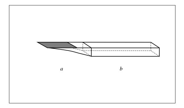
Figure 3. Application of a non-symmetric quadratic wedge-like damper covered by an absorbing film on one side (a) for suppression of flexural wave reflections from one of the edges of an elastic plate (b).
