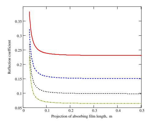
Figure 5. Effect of partial covering of a wedge by absorbing thin films on the reflection coefficient  $R_0$ : solid, dashed, dotted and dash-dotted curves correspond to the values of the film material loss factor v equal to 0.10, 0.15, 0.20 and 0.25 respectively; the value of the wedge truncation length  $x_0$  is  $2 \, cm$ , and the value of relative film stiffness  $\beta_2 = E_2/E_1$  is 0.2. Other parameters are the same as in Figure 4.
