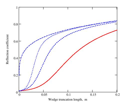
Figure 9. Effect of relative film stiffness  $\beta_2 = E_2/E_1$  on the reflection coefficient  $R_0$  for the wedge covered by a thick absorbing film: solid, dashed and dotted curves correspond to the values of  $E_2/E_1$  equal to 0.3, 0.03, and 0.003 respectively, dash-dotted curve corresponds to the uncovered wedge; the film thickness  $\delta$  is  $200 \ \mu m$ , other parameters are the same as on Figure 7.
