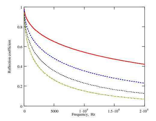
Figure 6. Frequency dependence of the reflection coefficient  $R_0$ : solid curve corresponds to the uncovered wedge, dashed, dotted, and dash-dotted curves correspond to wedges covered by thin absorbing films with the values of film material loss factor v equal to 0.05, 0.10 and 0.15 respectively. Other parameters are the same as in Figure 5.
