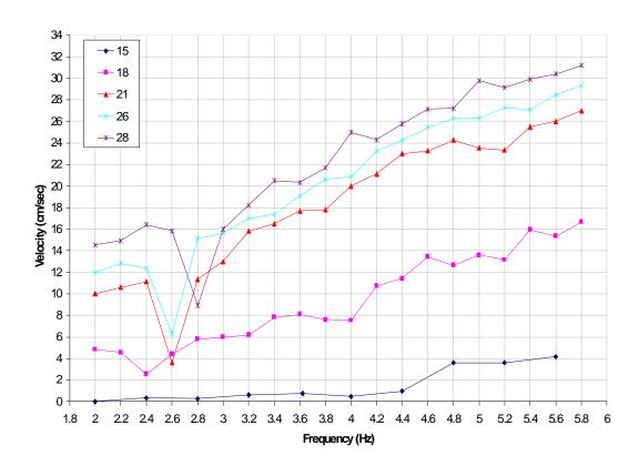
Fig. 6 Experimental values of steady state swimming speed of a model boat as functions of the propulsive wave frequency and amplitude (Krylov et al., 2010).
