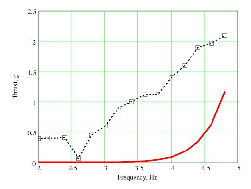
Fig. 10 Calculated thrust as a function of the propulsive wave frequency for the wave amplitude of 22 mm (solid line) in comparison with the corresponding experimental data (boxes) obtained for a mono-hull model boat (Krylov et al, 2010).
