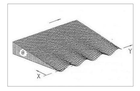
Fig. 1 Propagation of localised elastic waves along the tip of a linear wedge (Krylov, 1994).
