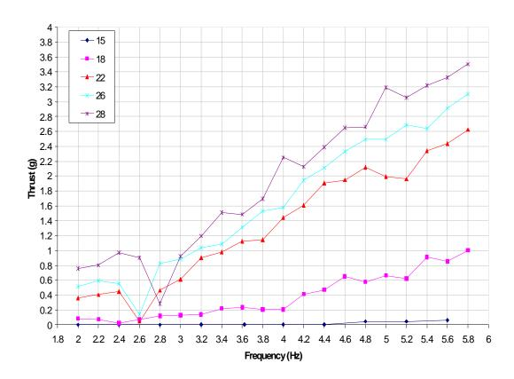
Fig. 7 Experimental values of generated thrust for a model boat as functions of the propulsive wave frequency and amplitude (Krylov et al., 2010).
