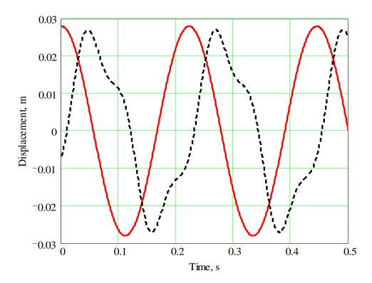
Fig. 8 Calculated waveform distortion of a localised flexural wave due to its nonlinear propagation at frequency f = 4.5 Hz and amplitude H = 28 mm along the tip of a rubber wedge immersed in water; calculations have been carried out for x = 0 (solid line) and for x = 0.17 m (dashed line).
