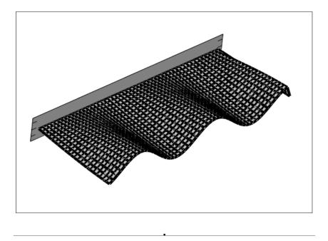
Fig. 2 Guided flexural waves propagating along the free edge of a clamped-free plate.
