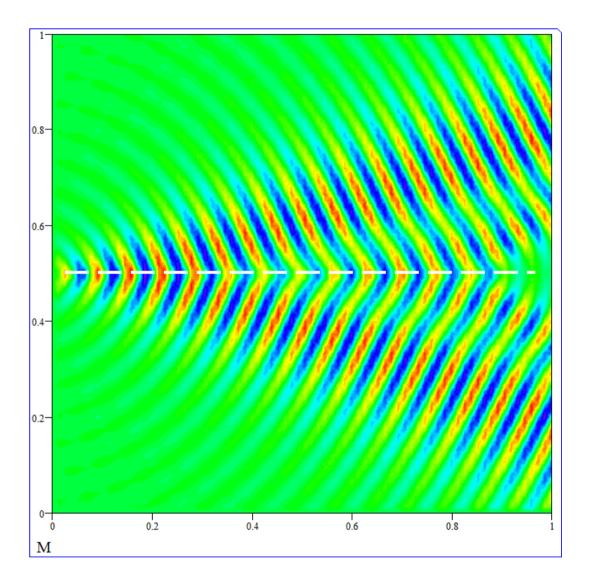
Fig. 10. Spatial distribution of ground vibrations (the same as in Fig. 9, but presented as a colour contour plot) generated by a single load travelling on a straight track (shown by a white dashed line) with acceleration  $a = 1 \text{ m/s}^2$  and initial train speed  $v_0 = 50 \text{ m/s}$ .
