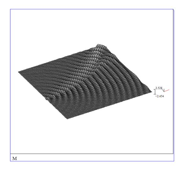
Fig. 5. Spatial distribution of ground vibration field (the same as in Fig.3, but presented as a greyscale surface plot) generated by a single axle load travelling at speed v = 50 m/s on a curved track with the radius of curvature R = 100 m.
