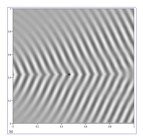
Fig. 7. Spatial distribution of ground vibration field (in arbitrary units, greyscale contour plot) generated over the area of  $75 \times 75$  m by a single axle load travelling at speed v = 50 m/s on a curved track with the radius of curvature R = 5000 m.
