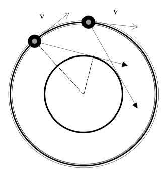
Fig. 1. Geometrical acoustics explanation of the focusing of Rayleigh waves radiated by a train (a single axle load in this example) travelling at speed v along a curved track of radius R under the condition of ground vibration boom ( $v > c_R$ ). The focusing occurs along the caustic line formed by a concentric circle of smaller radius r.
