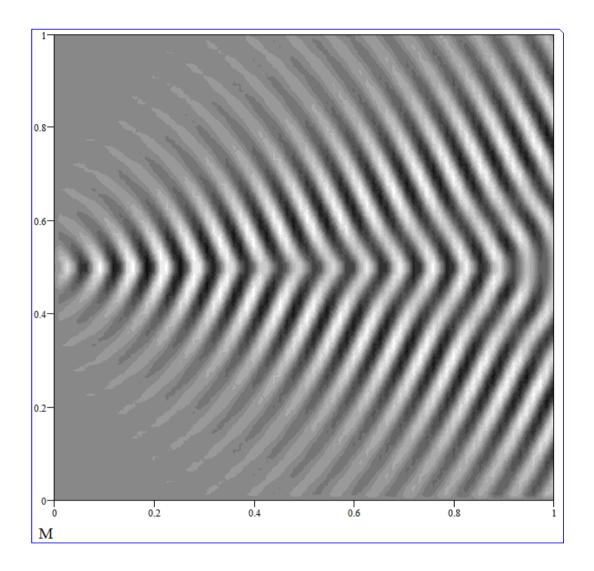
Fig. 11. Spatial distribution of ground vibrations (in arbitrary units, greyscale contour plot) generated over the area of  $75 \times 75$  m by a single load travelling on a straight track with acceleration a = 0.255 m/s<sup>2</sup> and initial train speed  $v_0 = 50$  m/s.
