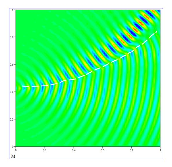
Fig. 4. Spatial distribution of ground vibration field (the same as in Fig. 3, but presented as a colour contour plot) generated by a single axle load travelling at speed v = 50 m/s on a curved track (shown by a white dashed line) with the radius of curvature R = 100 m.
