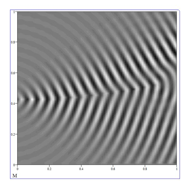
Fig. 6. Spatial distribution of ground vibration field (in arbitrary units, greyscale contour plot) generated over the area of  $75 \times 75$  m by a single axle load travelling at speed v = 50 m/s on a curved track with the radius of curvature R = 300 m.
