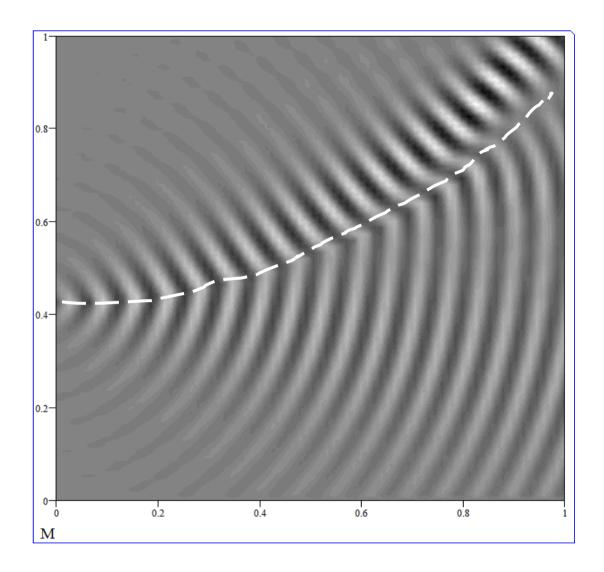
Fig. 3. Spatial distribution of ground vibration field (in arbitrary units, greyscale contour plot) generated over the area of  $75 \times 75$  m by a single axle load travelling at speed v = 50 m/s on a curved track (shown by a white dashed line) with the radius of curvature R = 100 m.
