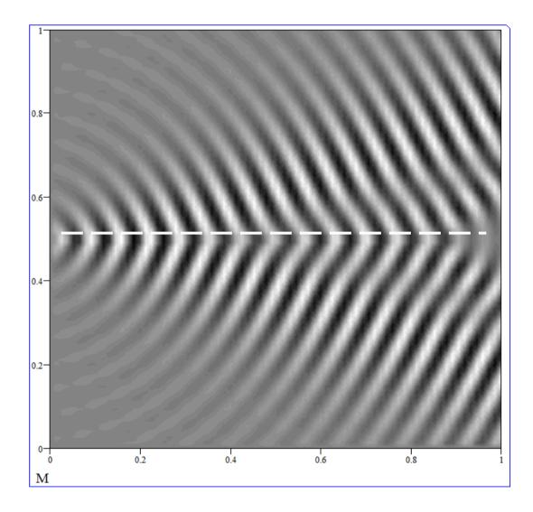
Fig. 9. Spatial distribution of ground vibrations (in arbitrary units, greyscale contour plot) generated over the area of  $75\times75$  m by a single load travelling on a straight track (shown by a white dashed line) with acceleration  $a = 1 \text{ m/s}^2$  and initial train speed  $v_0 = 50 \text{ m/s}$ .
