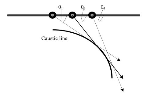
Fig. 8. Geometrical acoustics explanation of the focusing of Rayleigh waves radiated by a train (a single axle load in this example) travelling with constant acceleration a along a straight track under the condition of ground vibration boom  $(v > c_R)$ . The focusing occurs along the caustic line that is moving away from the track as the train passes by with acceleration.
