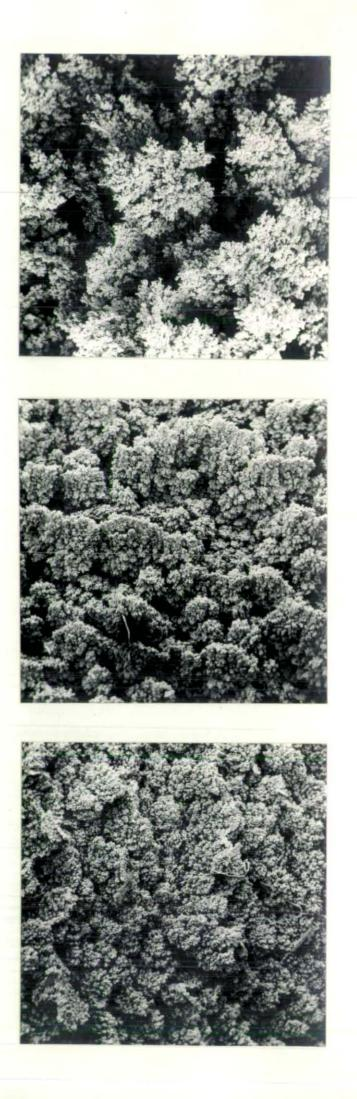
FIGS. 10.48 - 10.50 SCANNING ELECTRON MICROGRAPHS OF ROUGH COPPER DEPOSITS: SPECIAL FEATURES conditions generally as for FIG. 10.46 FIG. 10.48 MULTIPLE, LAYERED GROWTHS
