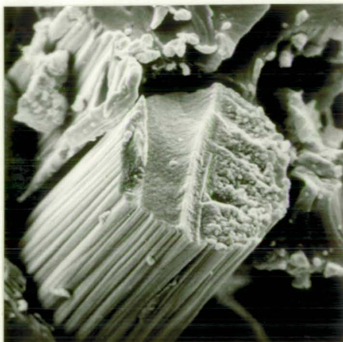
PLATE 25: A high magnification SEM micrograph of the end of a carbon fibre from a vinyl-ester CFRP compressive failure, 470-36 system. The fibre microbuckling failure has resulted in well defined tensile and compressive regions of fracture being visible
