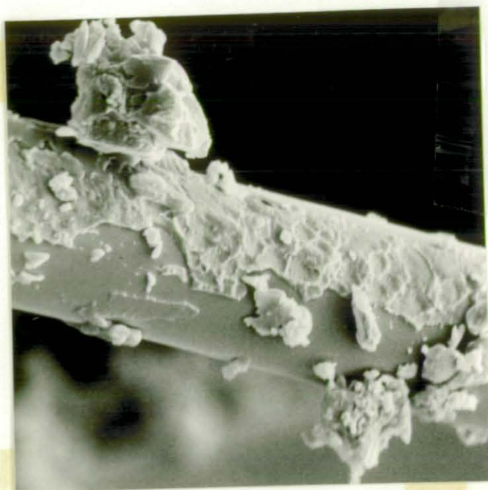
PLATE 22: A high magnification SEM micrograph of a fibre from an epoxy GRP transverse tensile failure, 913 matrix
