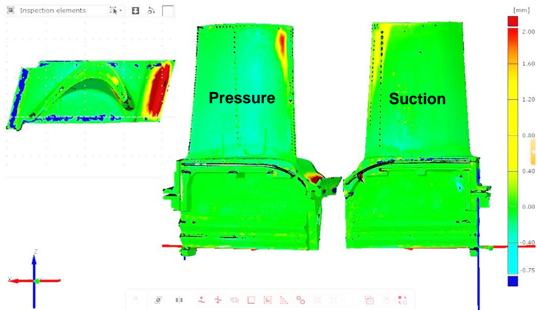
Figure 8.2. Dimensional comparisons of the ex-service run turbine blade before and after high temperature rejuvenation, showing top view, pressure side view and suction side view of the blade.
