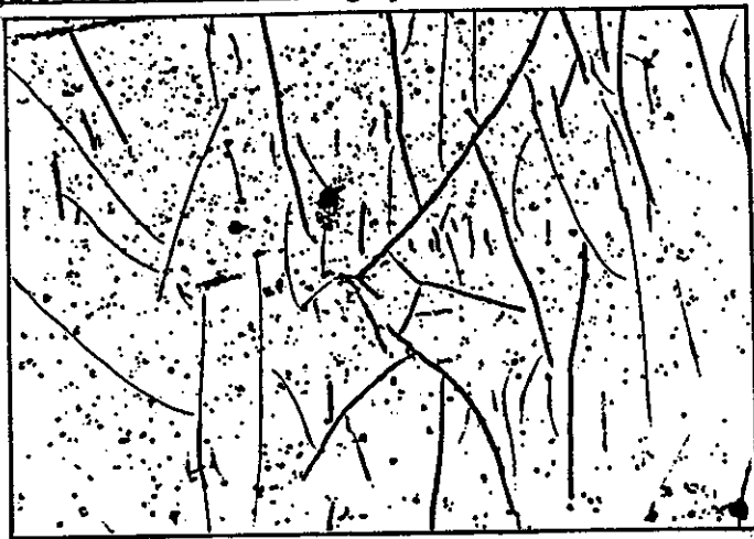
Figure 3.39: Surface Micrograph of PC-1, 3500hrs X-1200
