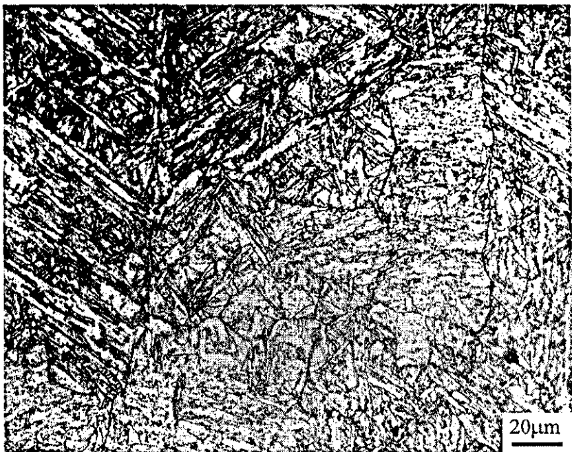
Fig. 6.9. Inhomogeneous WM microstructures in 5 # -1(P91)
