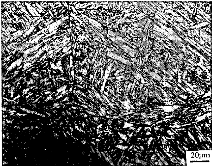
Fig. 6.29. Optical micrograph of parent metal of P92 (3#)
