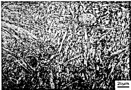
a) b) Fig. 6.31. Optical micrograph of parent metal of P122 (4 # ) a) cast side, b) forged side
