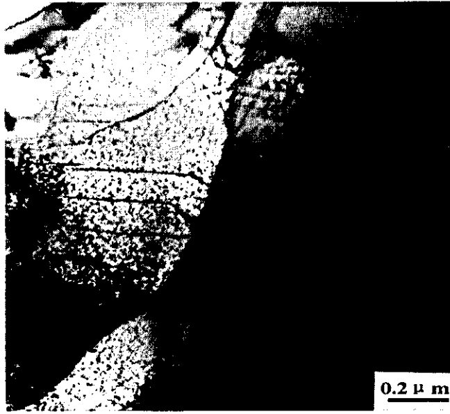
Fig. 6.39. Twin crystal martensite
