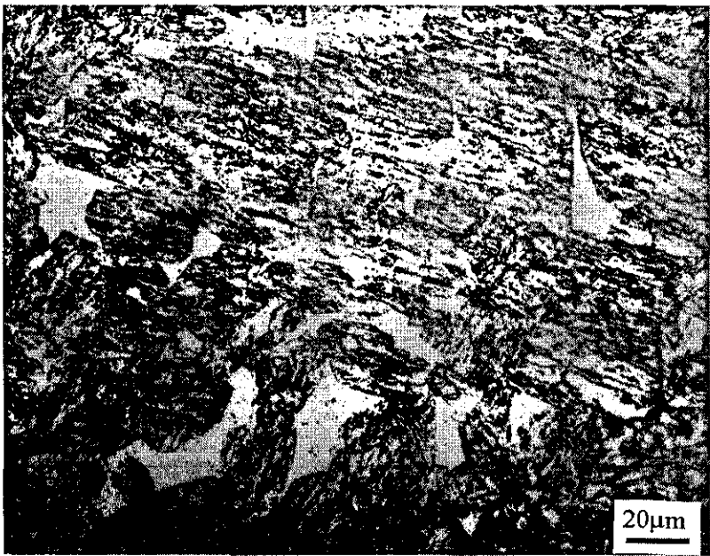
Fig. 6.4. The blocky ferrite in P92 weld(2 # )
