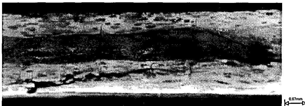
Figure 7.46 Photograph taper-line crack at 9J TIE for an intermediate impact from the three-box section.
