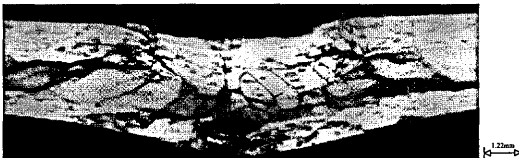
Figure 7.17 Photograph of collapsed upper CFM layer and considerable UD shear cracking under the impactor in 12J TIE shear coupon.
