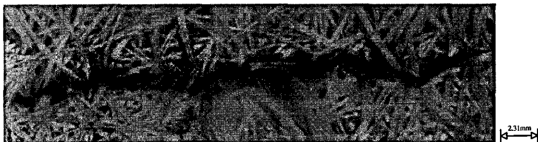
Figure 7.20 Photograph of lower CFM crack for the shear coupon from thermal deply exercise.
