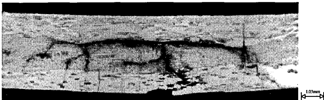
Figure 7.14 Photograph of lower CFM crack propagated through UD layer to promote upper interface delamination for 6.69J TIE shear coupon.
