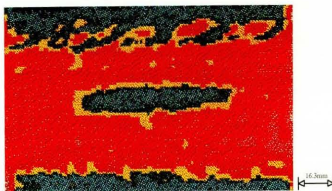
Figure 7.27 C-Scan plot from a 8J TIE transverse coupon (the attenuation along the edges are due to the tapers/webs and not damage).
