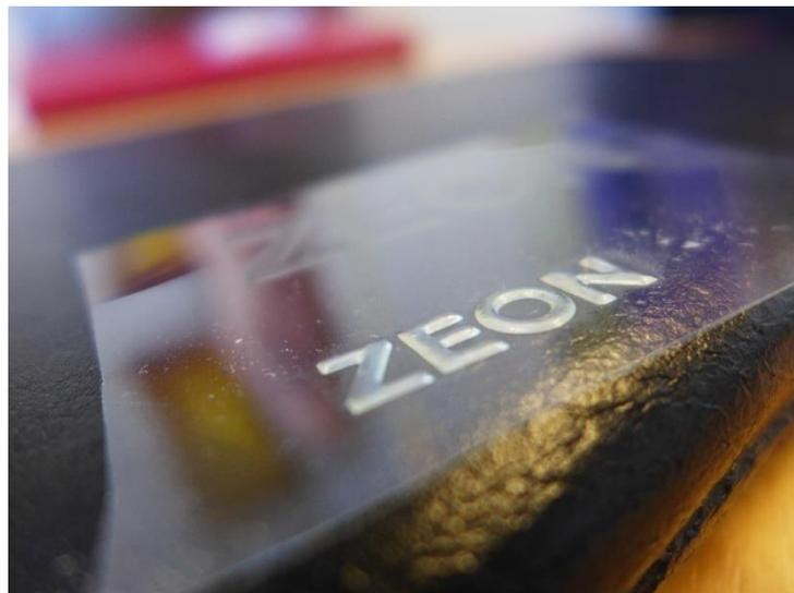
Figure 5.40 ZEON logo printed using HNBR liquid latex provided by Zeon Chemicals (approximately 4cm long and 1.5cm wide pattern)
