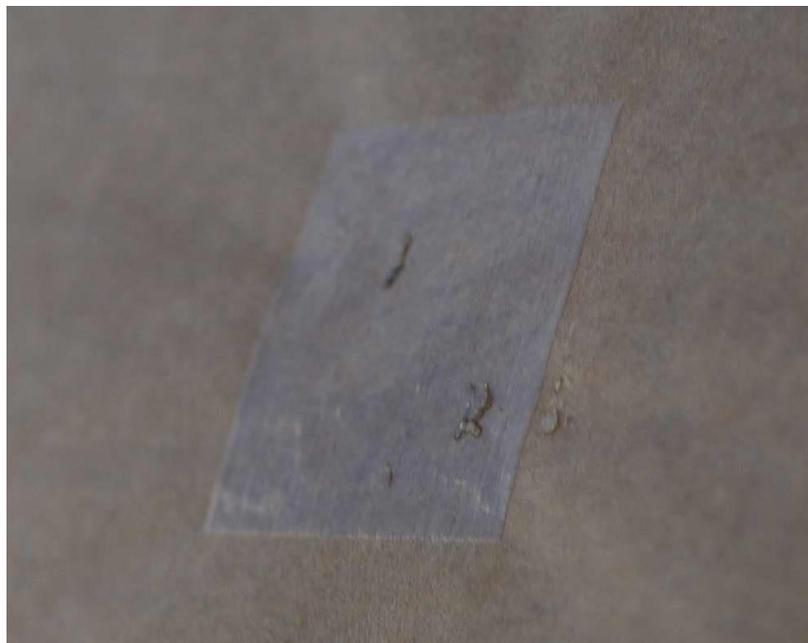
Figure 5.6 Photograph of 10 layers of diluted XSBR printed using a 2cm x 2cm square pattern onto silicone coated paper
