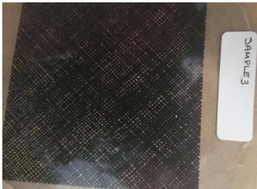
Figure 6.4 A crosshatch pattern (3 layers) printed onto cast sheet of XSBR latex
