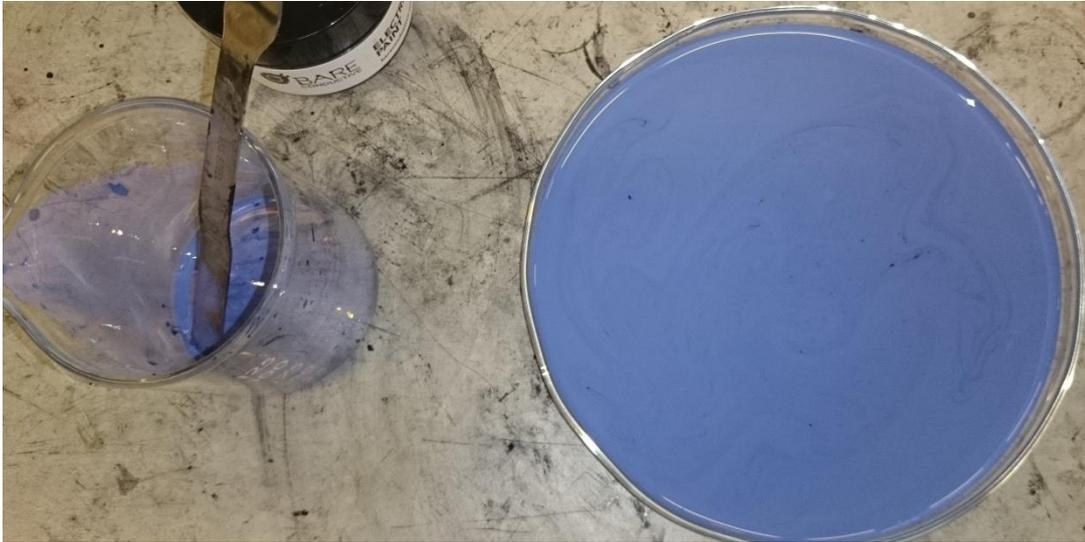
Figure 5.69 XSBR combined with carbon black in a petri dish to be dried
