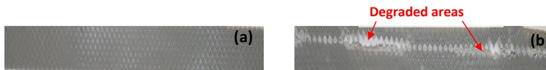
Fig.1. Segments of silicone rubber gaskets (a) unused (b) after 8000 h used in the fuel cell
