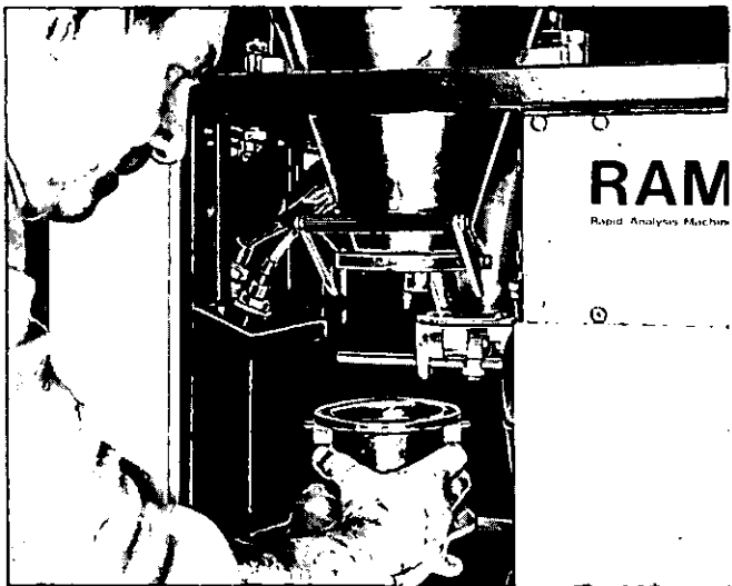
5 Constant volume vessel is removed and weighed.
