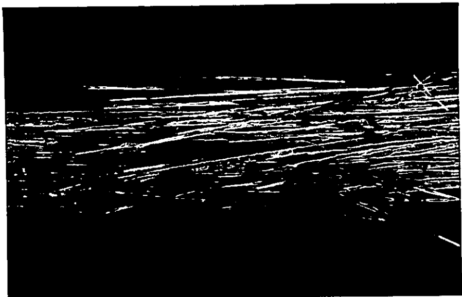
c) Fracture surface of 913 (conditioned at 95% and water bath)
