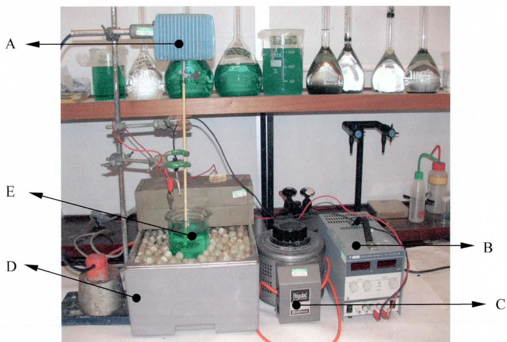
Figure 6.2 Photograph of the experimental apparatus showing (A) Vibromixer (B) Power supply unit (C) Variac motor (D) Water bath (E) Electrolyte with submerged agitator disc.
