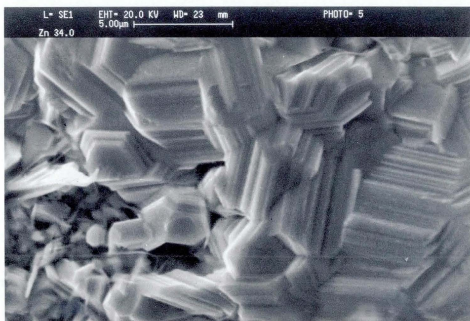
Figure 7.8 SEM micrograph of zinc electrodeposit from the acid bath. Current density 3 A/dm 2 , agitation 800 rpm and pH 5.
