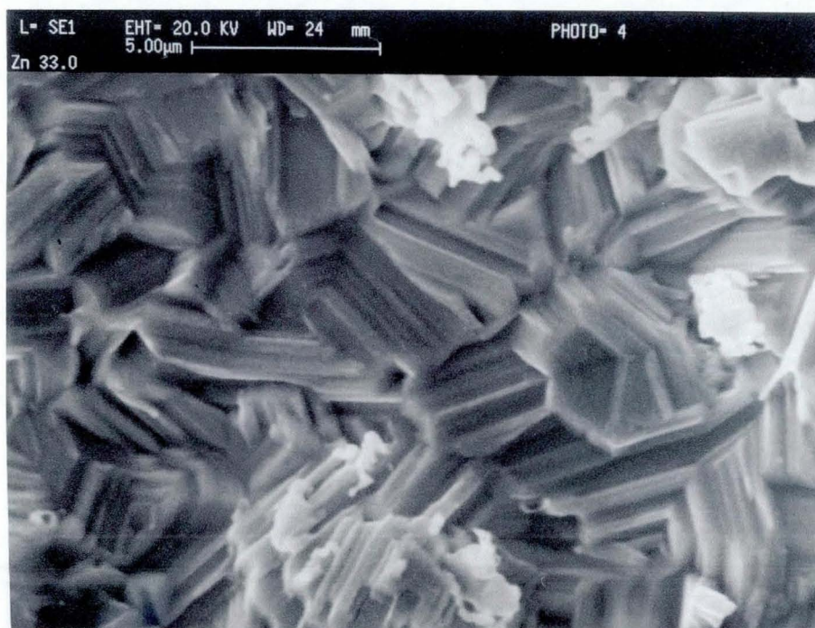
Figure 7.10 SEM micrograph of zinc electrodeposit from the acid bath. Current density 3 \text{ A/dm}^2 , agitation 800 rpm, pH 2, T = 40 \text{ }^\circ\text{C} .
