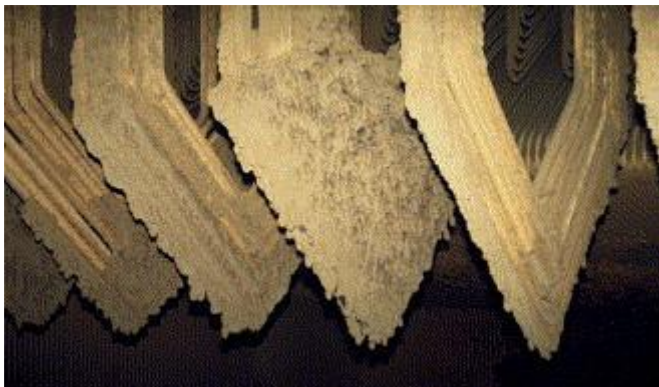
Figure 2-7a: Deposit formation in the superheater region of the Amager power station co-firing straw and coal 60
