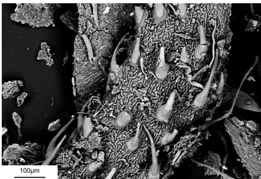
Figure 4-2: Electronmicrograph of raw hemp fuel showing a clear organic matrix i.e. the fibrous nature, with trichomes, large silicate structures attached
