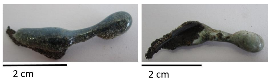
Figure 6-32: Glassy slag flow removed from EUC E
