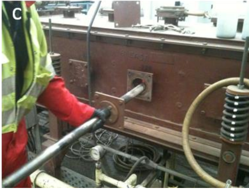
Figure 3-1c: Ceramic probe inserted into the combustion rig to collect deposits
