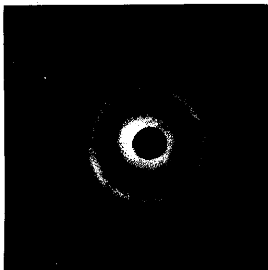
FIGURE 4E3. 1(a). X-ray photograph of polyurethane based on Capa 220 : H 12 MDI : 1,4 BD at 1:3:2 block ratio
