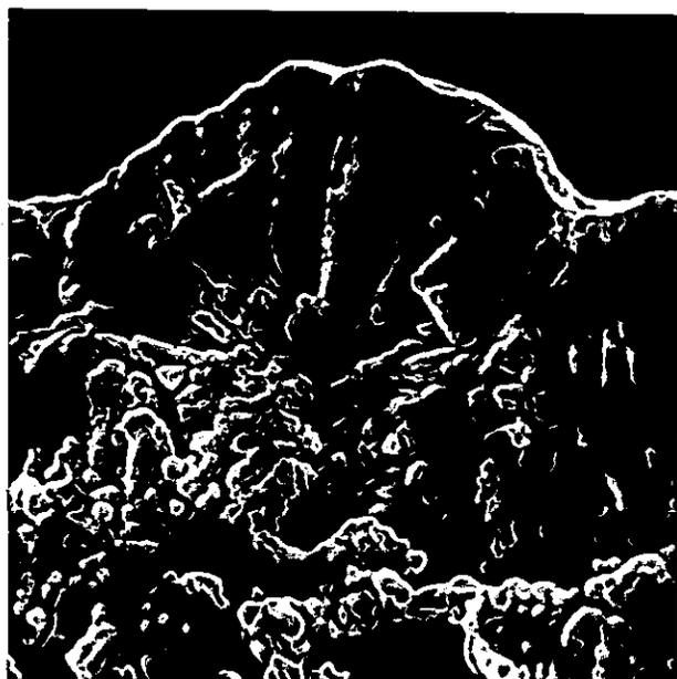
Figure 4.18 Fracture surface of C.V.D. TiN coating on an as-coated insert showing coating structure associated with surface protrusion. S.E.M. x 7000.
