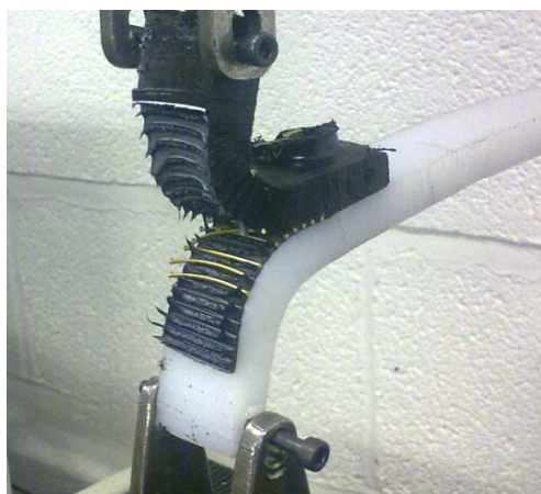
Figure 5-34 EF peeling test followed by ductile failure
