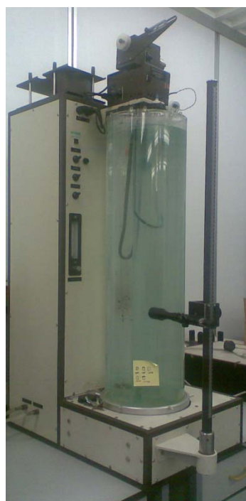
Figure 3-6 Schematic of density gradient column and filling device [123]
