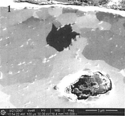
Figure 8.6: Ion beam induced secondary electron images of the creep specimen (after rupture) with the parent metal supplied in the pre-aged condition (C). The image on the right is a secondary electron image showing the position of the ion beam images below from the Type IV crack (position 1) progressively towards the parent metal region.
