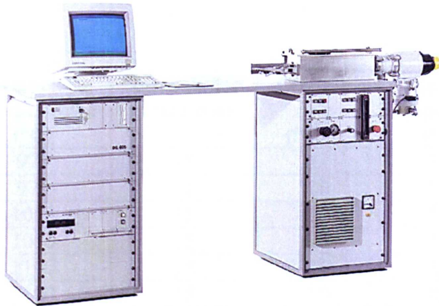
Figure 3.3: Baehr-Thermoanalyse DIL805 dilatometer. From Baehr Thermoanalyse product website [96] .
