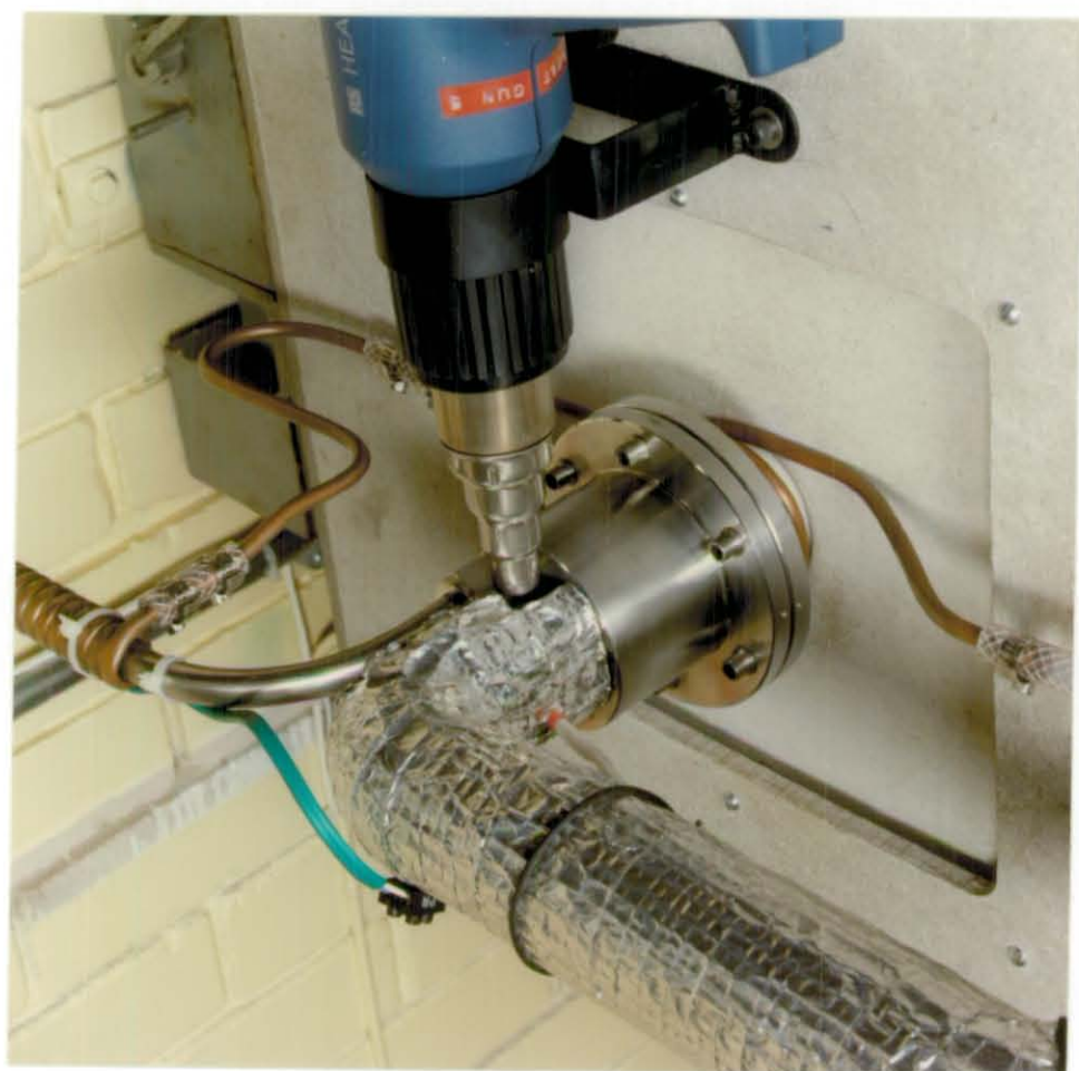
Figure 3.9 Inlet end of reactor coating chamber - detailed view
