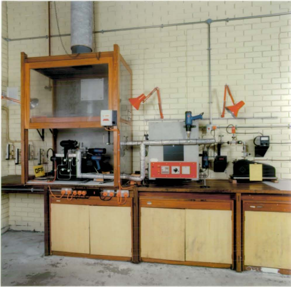
Figure 3.13 View of complete laboratory-scale Al 2 O 3 CVD reactor
