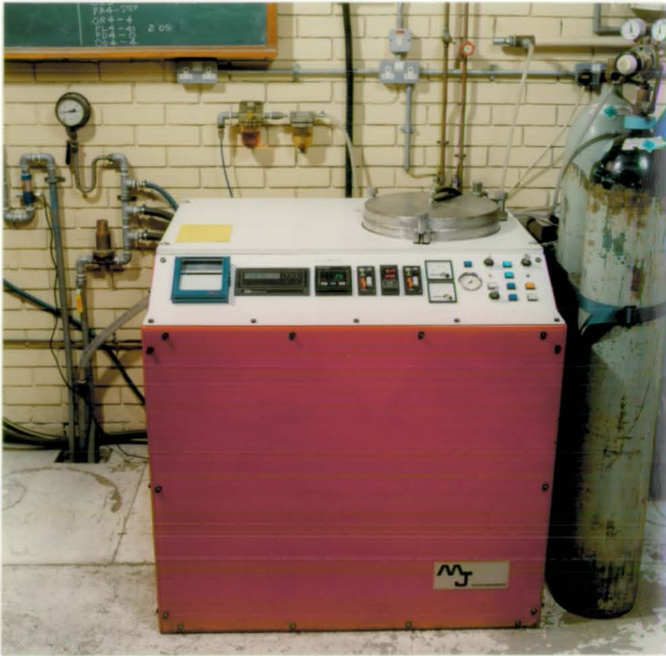
Figure 3.16 Vacuum heat treatment furnace
