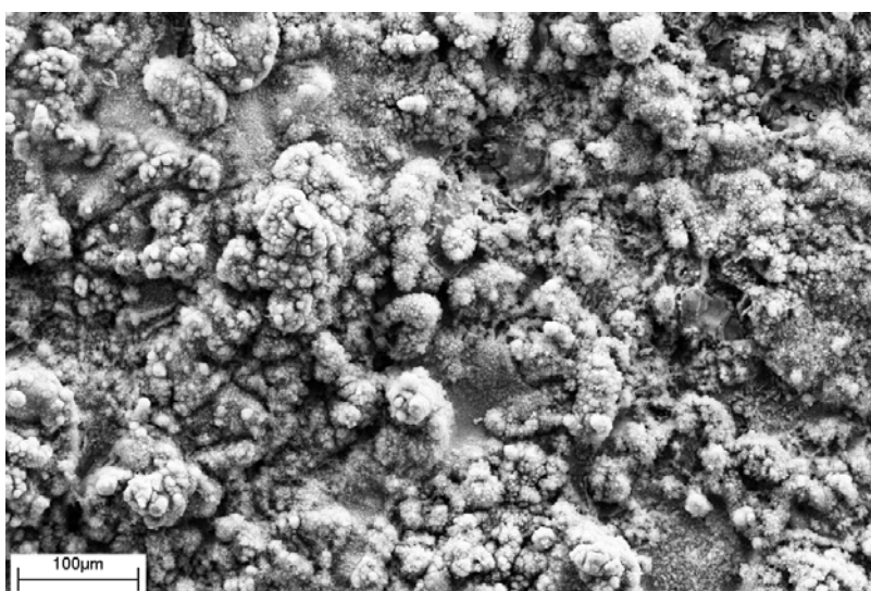
Figure 69. SEM secondary electron micrograph of the surface of the EC coating after porosity testing together with an elemental compositional analysis using EDX below
