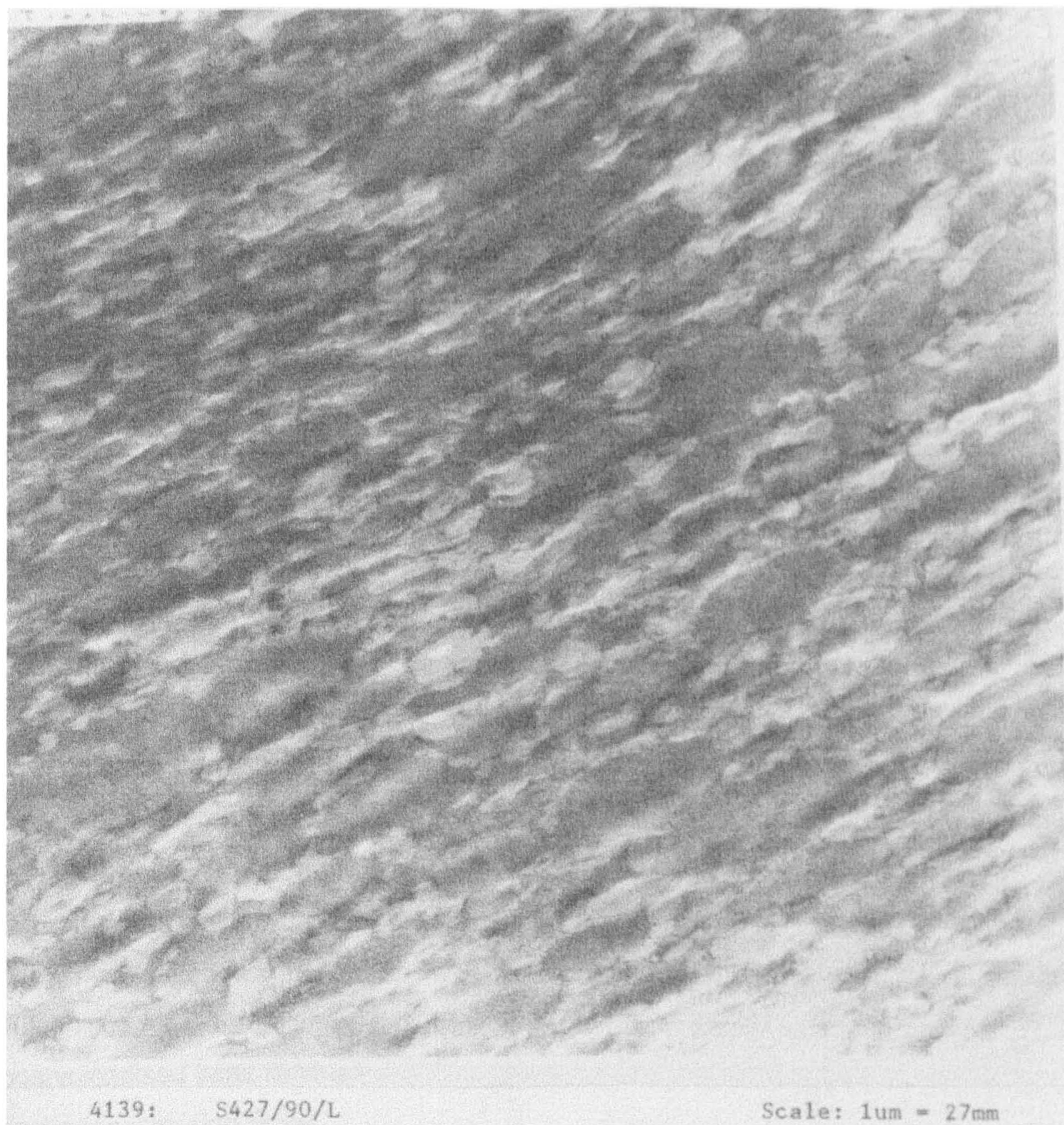
Figure 79 Compounded Latex Film Heated for 90 min at 90°C followed by Aqueous Leach 24 h at Room Temperature (preparation A(31))
