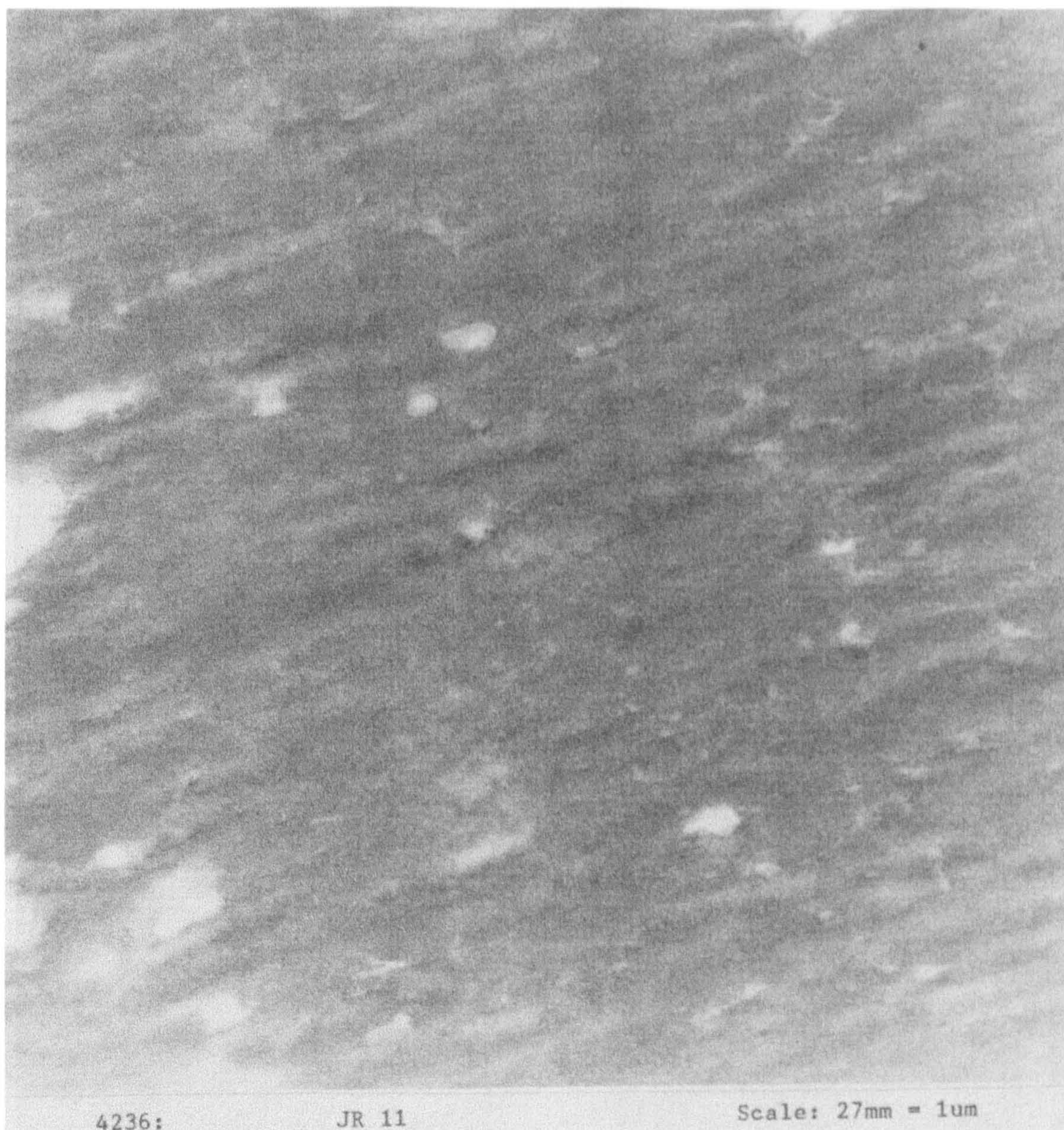
Figure 74 Compounded Latex Film Heated for 30 min at 130°C (preparation A(33))
