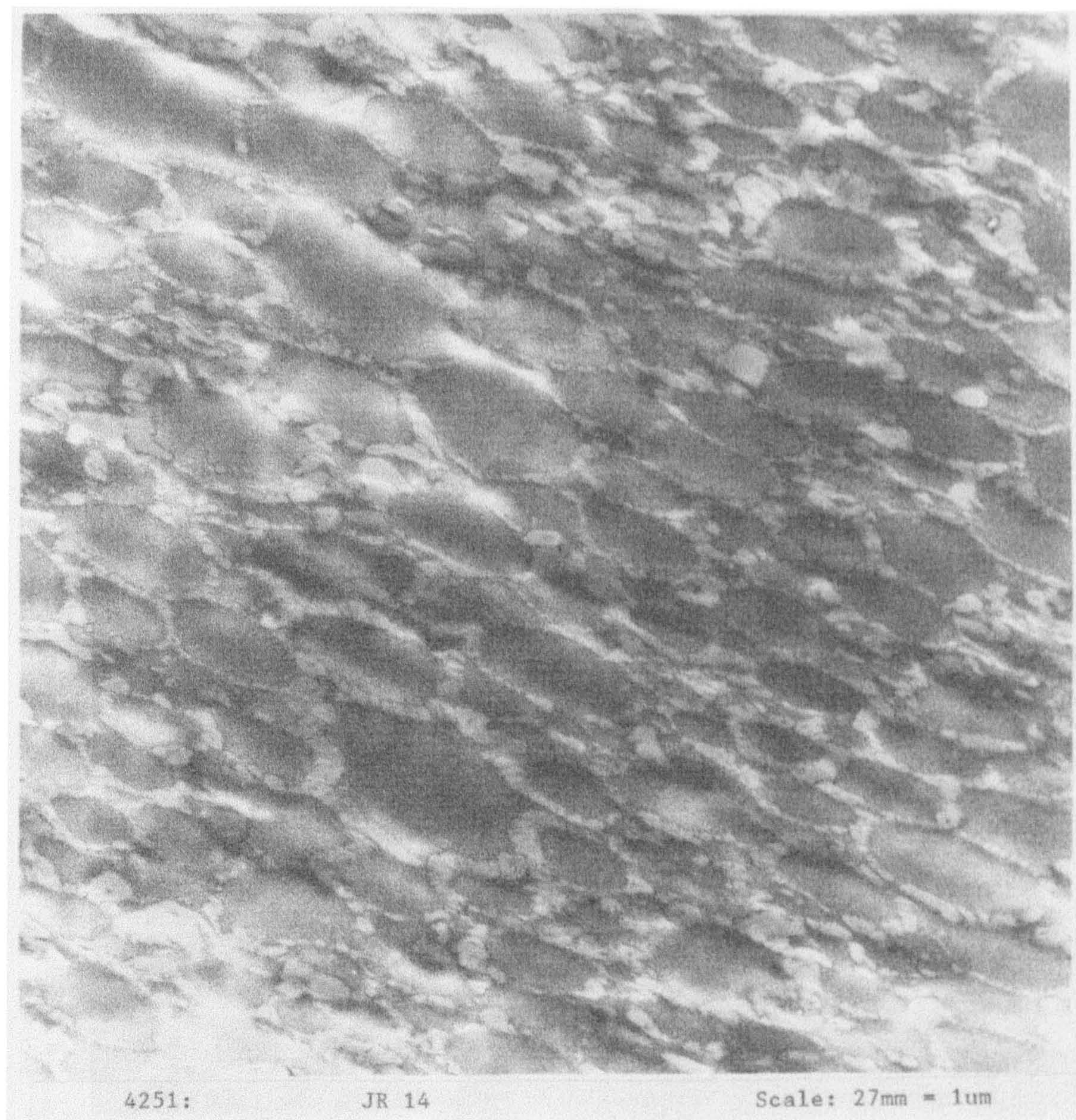
Figure 70 Compounded Latex Film Heated for 5 min at 130°C (preparation A(32))
