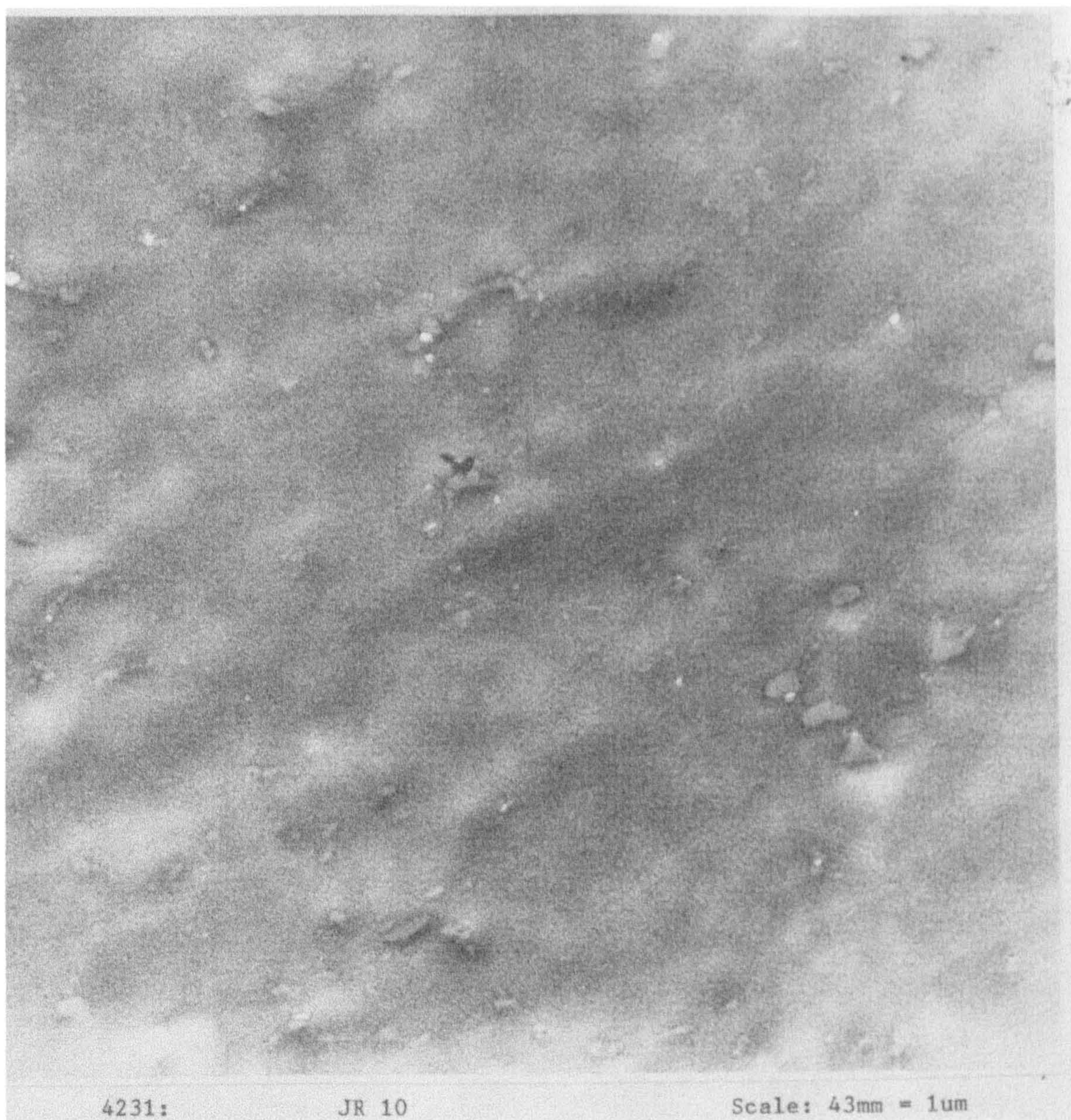
Figure 73 Compounded Latex Film Heated for 20 min at 130°C (preparation A(33))
