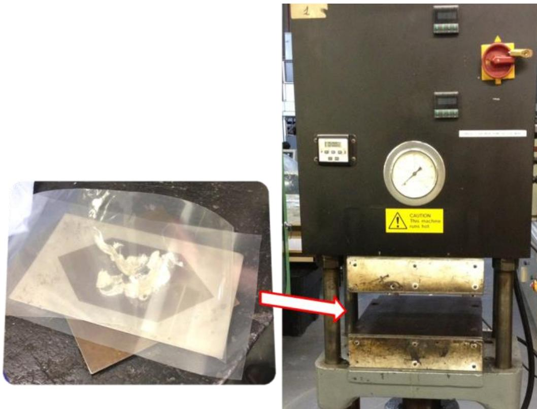
Figure 3.2 Compression moulding sample setup and hot press machine
