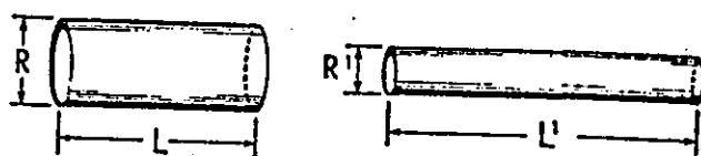
FIGURE 3.3: TYPES OF STEADY ELONGATIONAL DEFORMATION 56
