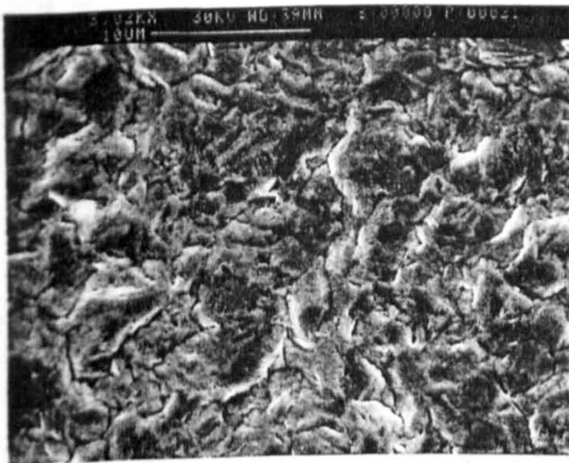
Figure 29. A gold deposit from a citrate electrolyte produced under conventional conditions. C.D. 5.0 mA/cm 2 , 0.06M gold, Thickness 18 μm.
