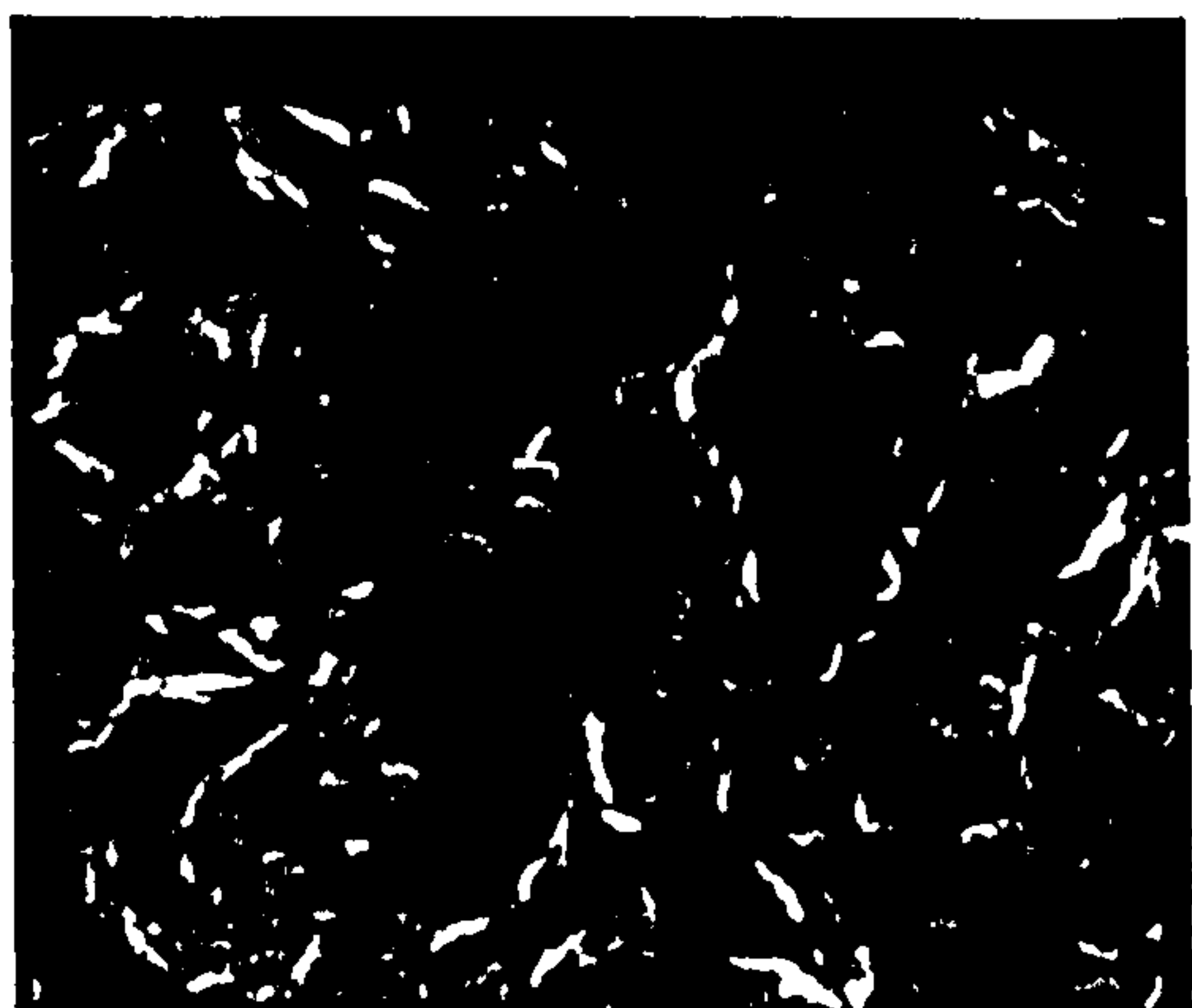
Fig.4: Gold deposit produced from a citrate gold electrolyte by conventional deposition C.D. = 5 \text{ A/cm}^2 ; 0.06M gold; Thickness = 18 \text{ μm}
