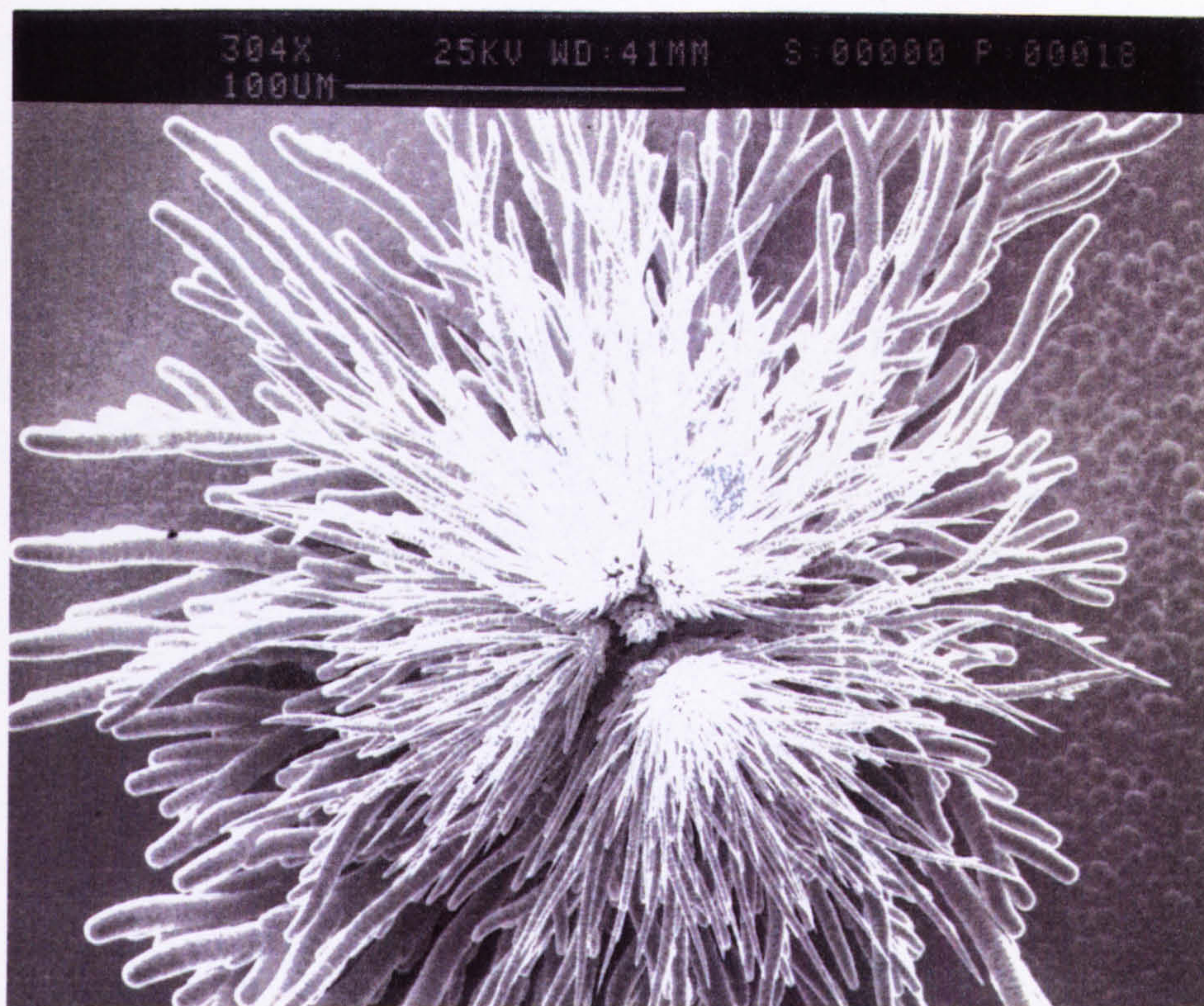
Photograph 19. The effects of electrolyte velocity. 0.28M citrate electrolyte. Current density = 4.75 \text{ A cm}^{-2} . Temp. = 55^{\circ}\text{C} . Re. = 1044.
