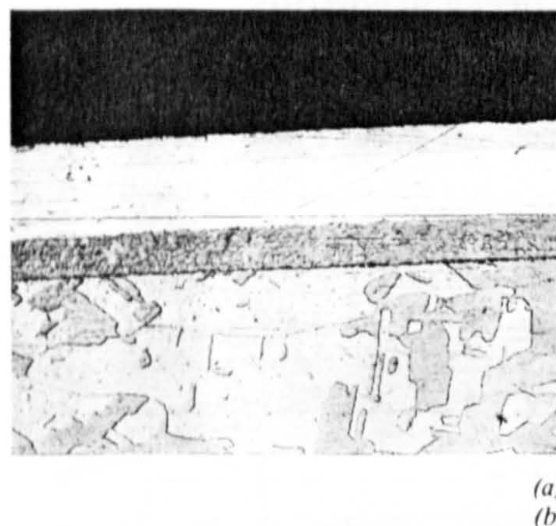
Figure 2. (a) Microsection of a copper deposit, X 1000. (b) Surface Morphology of the same deposit. 0.8M copper, C.D. 2.0 A/cm 2 , Re. 1365.
