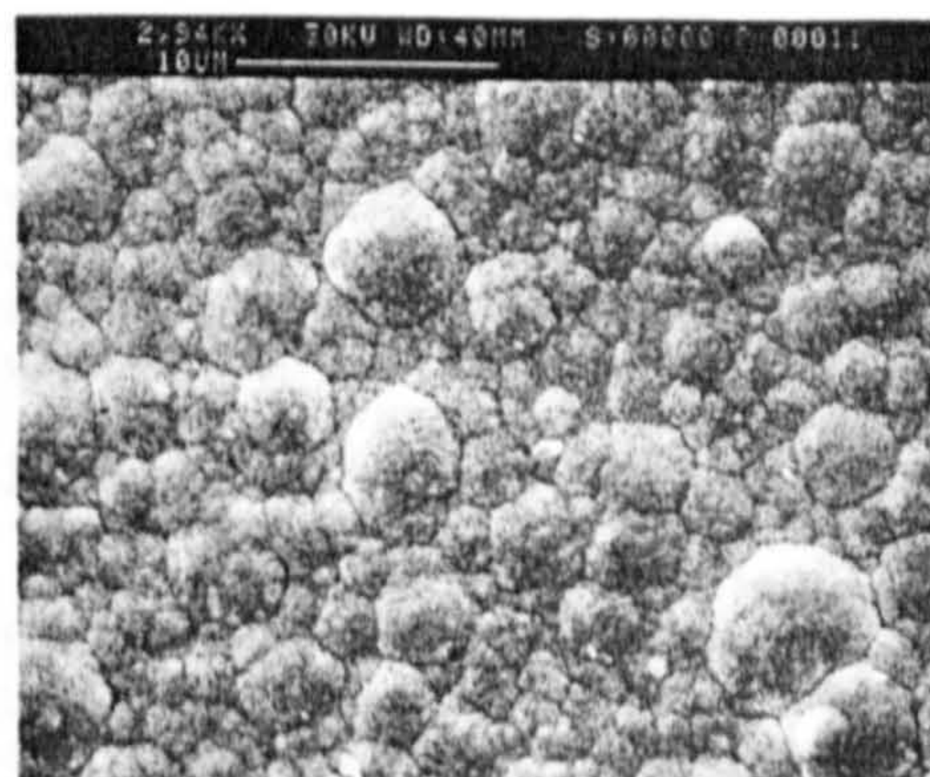
Figure 19. The morphology of the gold deposit produced at the greatest plating rate. 0.17M gold (citrate electrolyte). Temp. 55^\circ\text{C} C.D. 6.0 \text{ A/cm}^2 , Re. 12,078, plating rate 3.4 \mu\text{m/sec} , pH 8.1.
