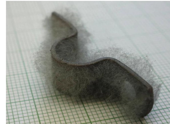
Many long zinc whiskers on zinc coated steel [1]
