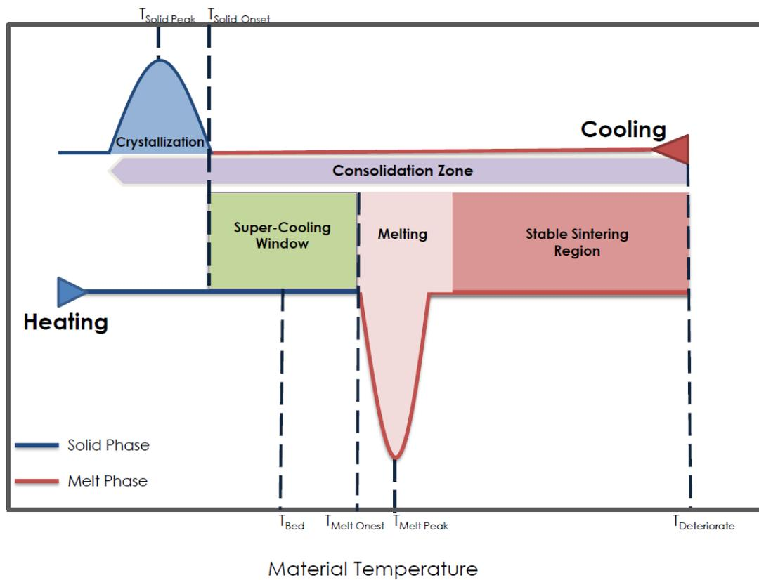
**Figure 7 Laser sintering window, for semi-crystalline polymers**
