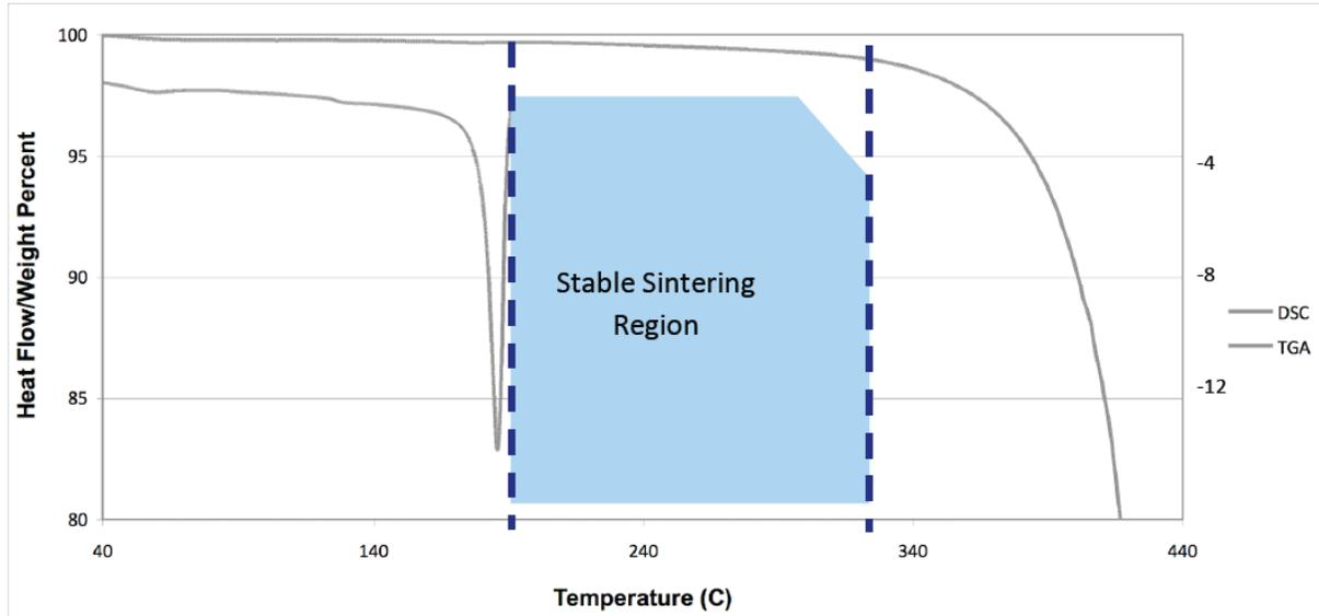
**Figure 6 ‘Stable sintering region’ proposed for semi-crystalline polymers**
