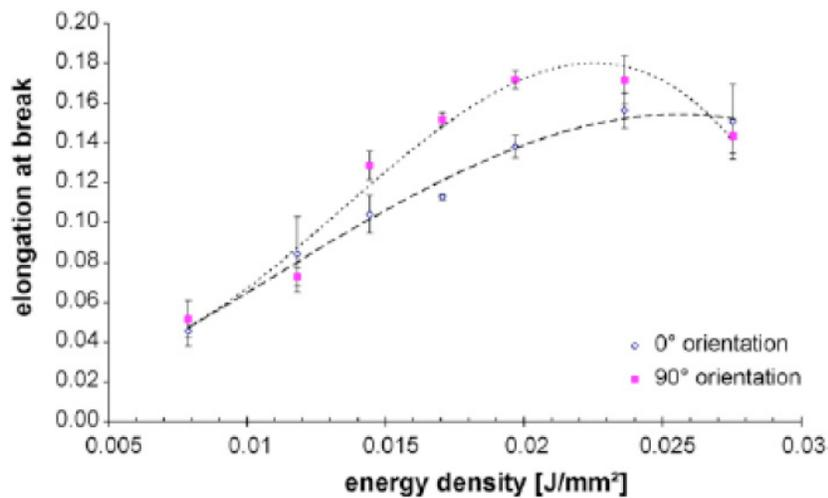
**Figure 1 Effect of laser power on elongation at break in Nylon-12 (Caulfield 2006)**
