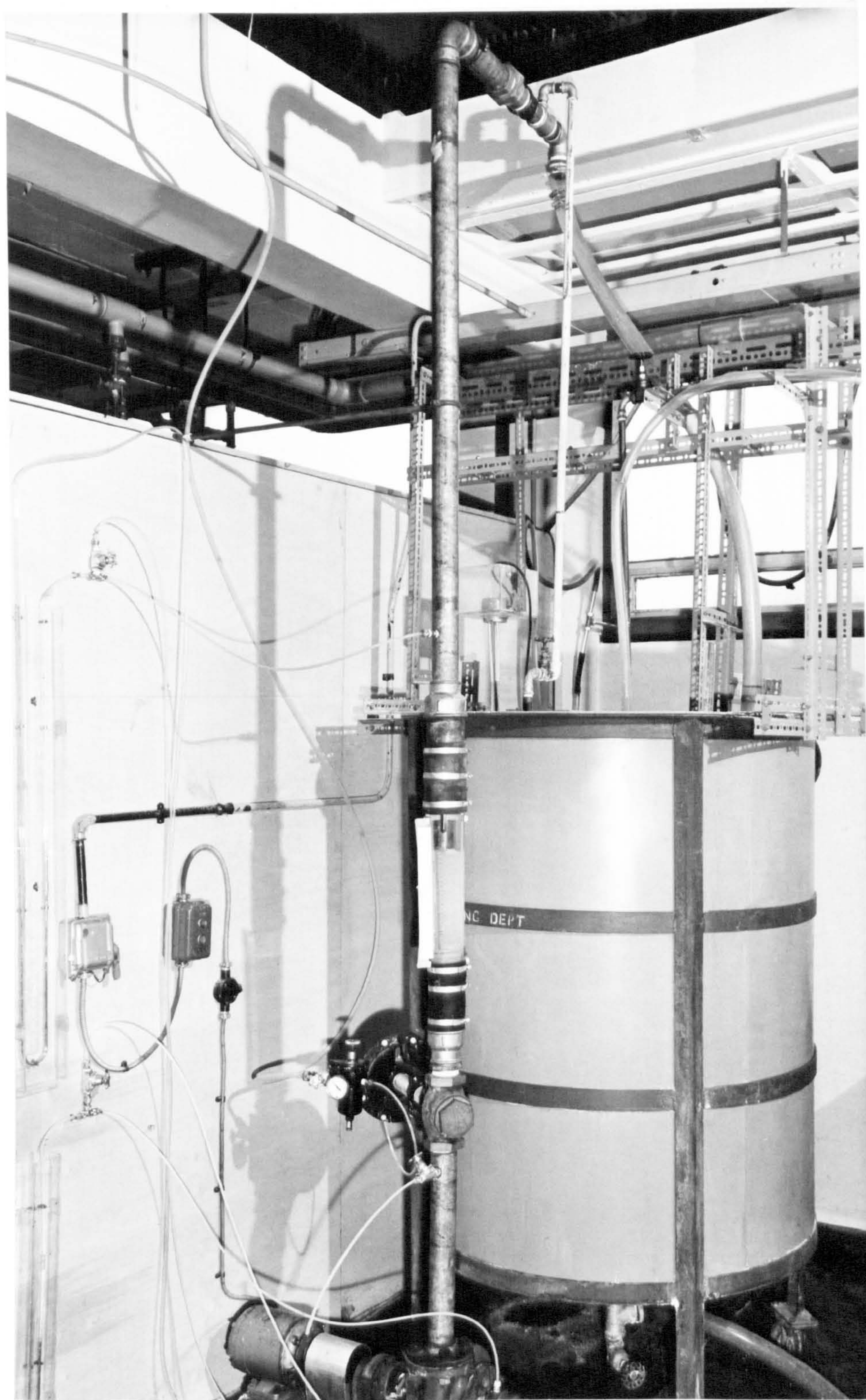
PLATE II. Experimental set up for plunging jet aeration experiments.
