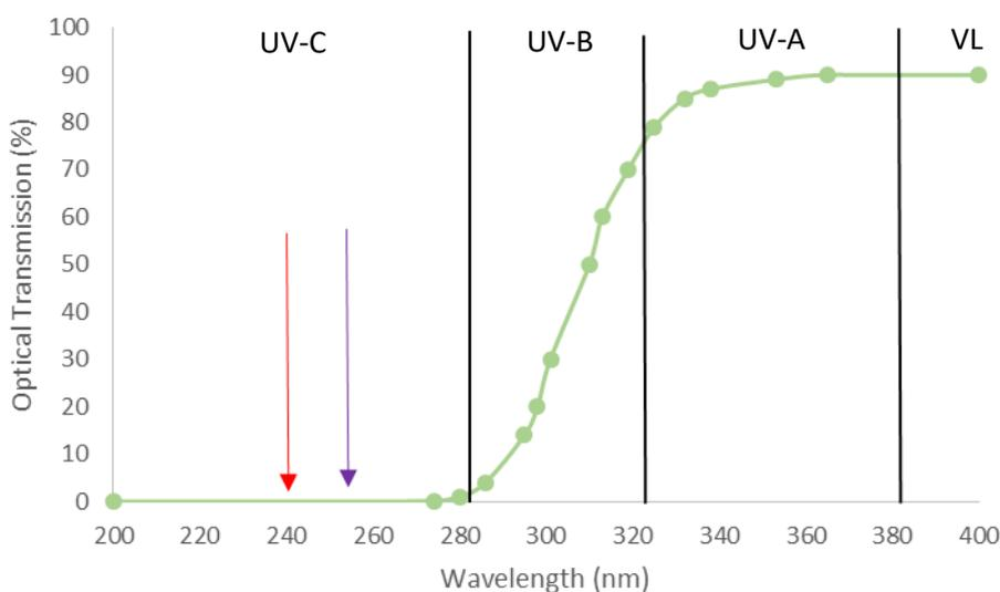
**Figure 6.1:** Optical transmission for the Borofloat<sup>®</sup> 33 UV-C filtering glass (Schott). The red arrow indicates the optical cut off point (minimum wavelength) emitted by the high-intensity, pulsed polychromatic light source. The purple arrow indicates the standard peak emission for low-intensity UV-C sources (254 nm). Vertical lines indicate the groups of electromagnetic radiation UV, groups C, B and A along with VL (visible light).
