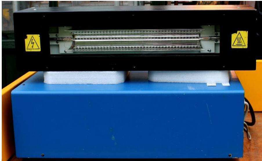
**Figure 2.2:** The high-intensity, pulsed polychromatic light source with light source LH-840 and RT-847 cabinet with inbuilt RC-802 controller (XENON).
