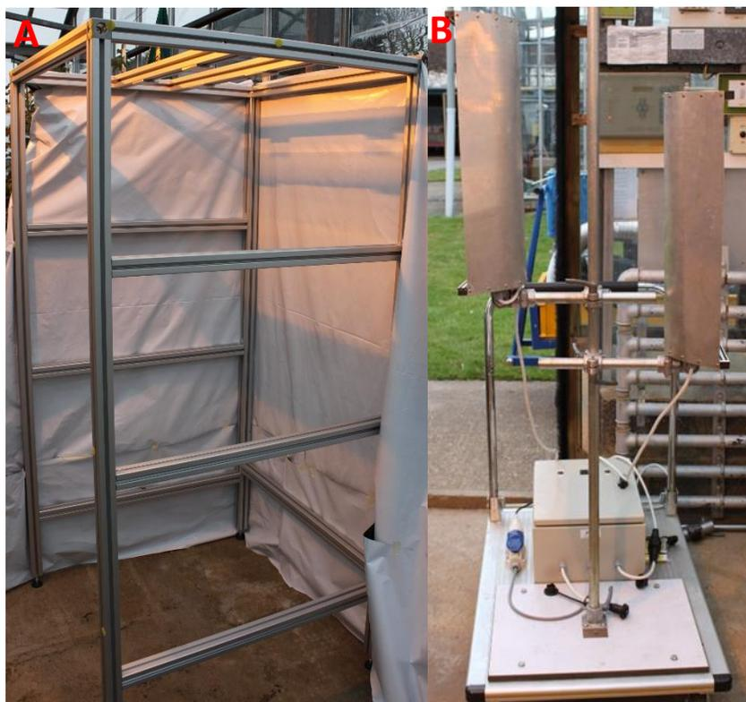
**Figure 2.1:** The enclosed gantry in which treatments were performed (A) and the low-intensity UV-C source with two separate sources mounted in parabolic reflectors (B).
