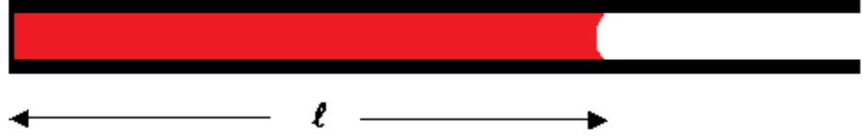
Figure 4A.1: Capillary imbibition of a non-Newtonian liquid into a thin capillary.
